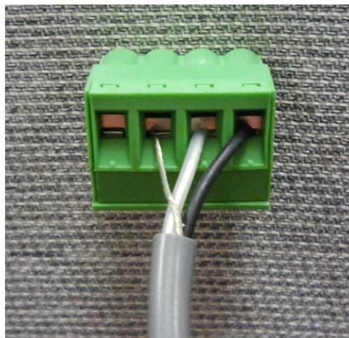
Figure 10 - Four-Terminal Phoenix Connector
