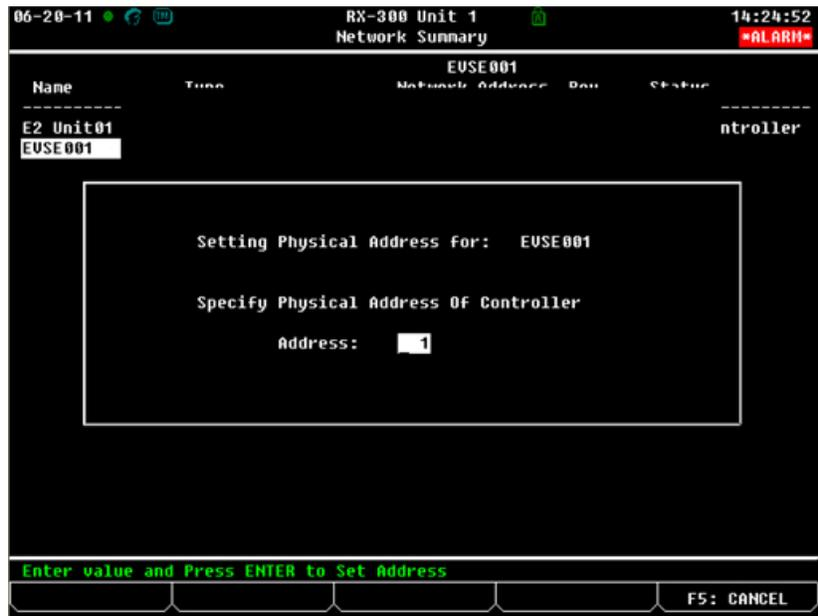
Figure 9 - Device Physical Address Setting
