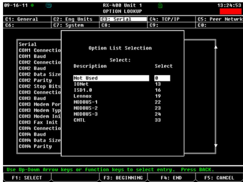
Figure 4 - Option List Selection Screen - Connection
