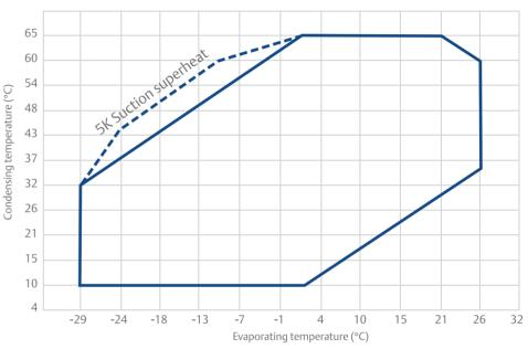
Based on: 11.1K SH, 8.3K SC, 35.0 C Ambient (Solid line boundaries) Refer to application engineering bulletin for details on the speed range throughout the operating envelope.
