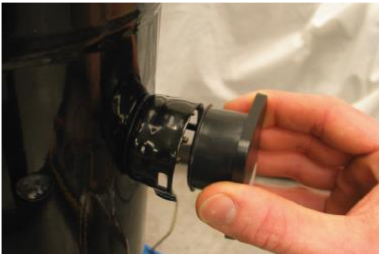
Figure 15: Moulded plug used for cable connection to the compressor
