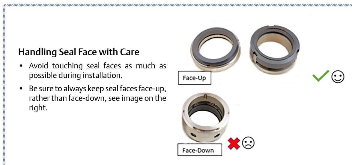
Figure 5-51. Handling Seal Face with Care
