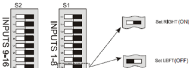
Input Type Dip Switches for MultiFlex or 16AI Board
