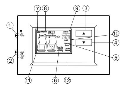
Whenever "I Replace" appears in the display, new premium brand AA alkaline batteries should be installed. If the house will be unoccupied for an extended period and either "I replace" is displayed, install new batteries before leaving.
