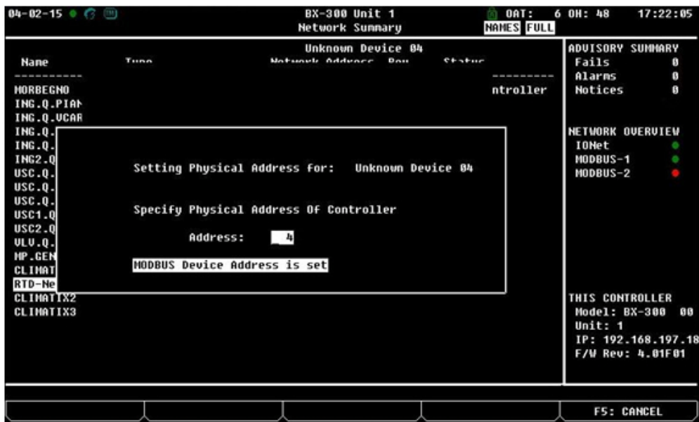
Figure 9 - MODBUS Device Address Setting
