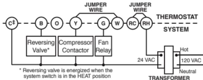
Typical wiring diagram for heat pump
