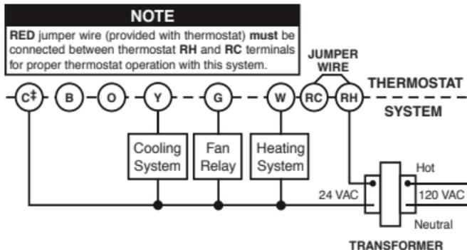
Typical wiring diagram for heat/cool,
