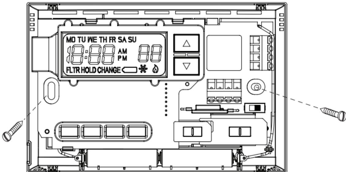
Mount your new thermostat base using the supplied screws. Drill holes and insert wall anchors to secure the thermostat base to the wall, if necessary.
