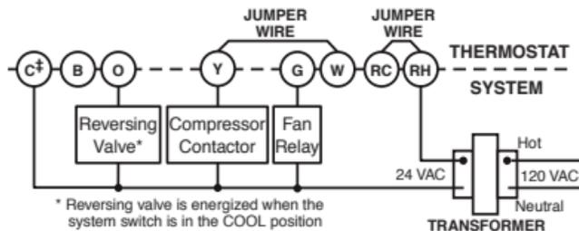
Typical wiring diagram for heat pump
