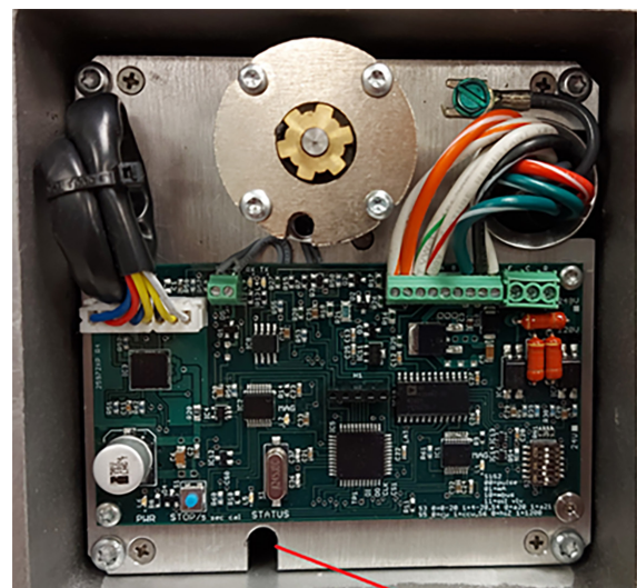
Figure 4-4. Rotation Check. Motor/Brake Shaft Spins Opposite of the Command Shaft
