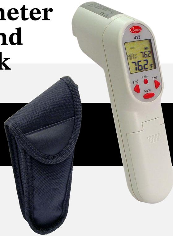
The 412's innovative design incorporates a non-contact infrared thermometer with laser sight to measure surface temperatures with distance to spot ratio of 12:1 and backlit LCD for easy temperature viewing. The type K thermocouple jack accepts all type K probes. Use an insertion probe to measure internal temperatures.
