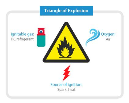
An additional condition is required for explosion. The mixture of released flammable refrigerant from the refrigeration system and air in atmosphere must be within a certain mixture range.
