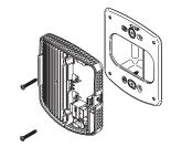
Place the thermostat cover back onto the base hinge and close cover. Install screw to secure cover.
