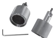
The manual tool should always be ordered with any ICM/ICAD assembly. This tool gives the user the ability to remove the ICAD actuator and manually rotate the valve in the open or close direction depending on need and application. When using the manual tool, a clockwise rotation will open the valve and a counter-clockwise rotation will close the valve.
