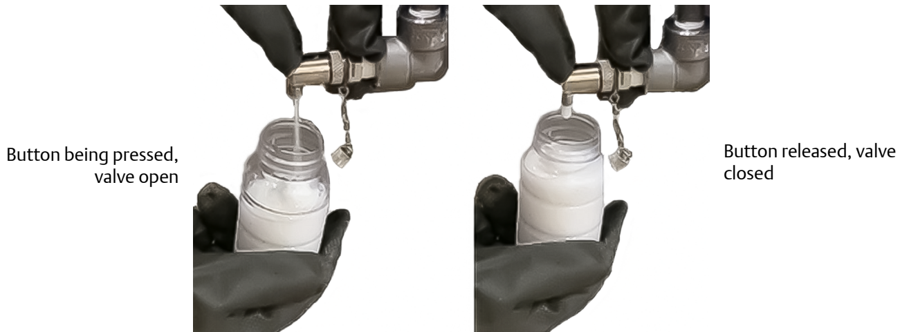
Figure 5-5. Operating the Oil Sampling Valve
