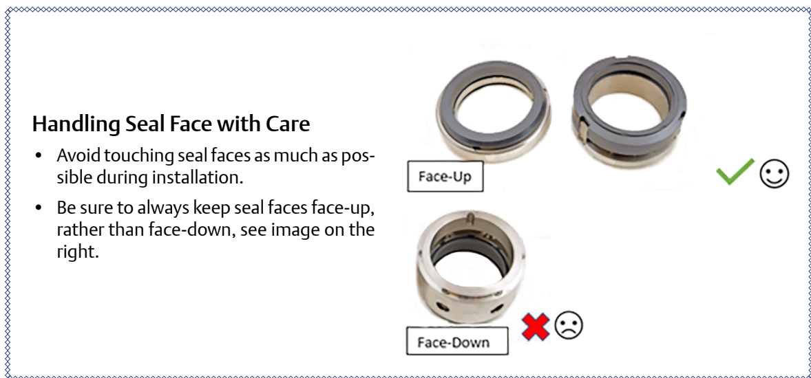
Figure 5-40. Handling Seal Face with Care
