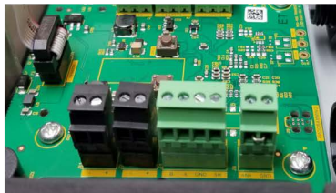
Analog output terminal block installed with jumper
