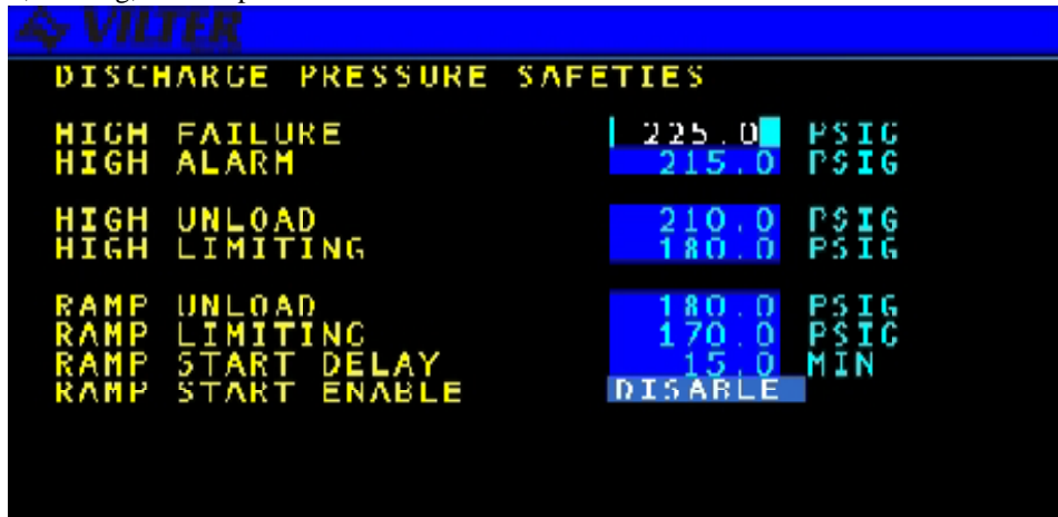
Discharge Pressure Setpoints Data Entry Screen
