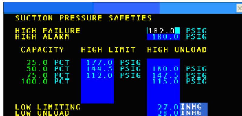
High Suction Pressure Setpoints Screen
