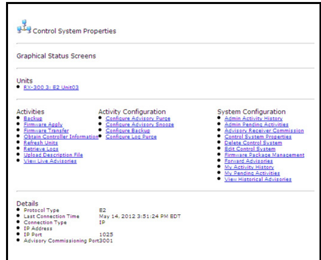
Figure 5-14 - Control System Properties Page
