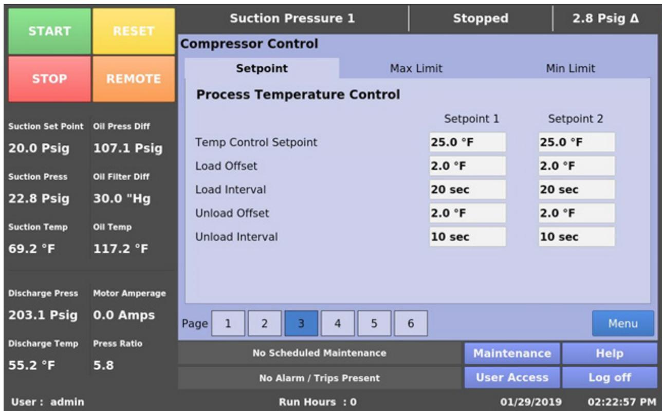
Figure 5-2. Compressor Control Screen - Process Temperature Control
