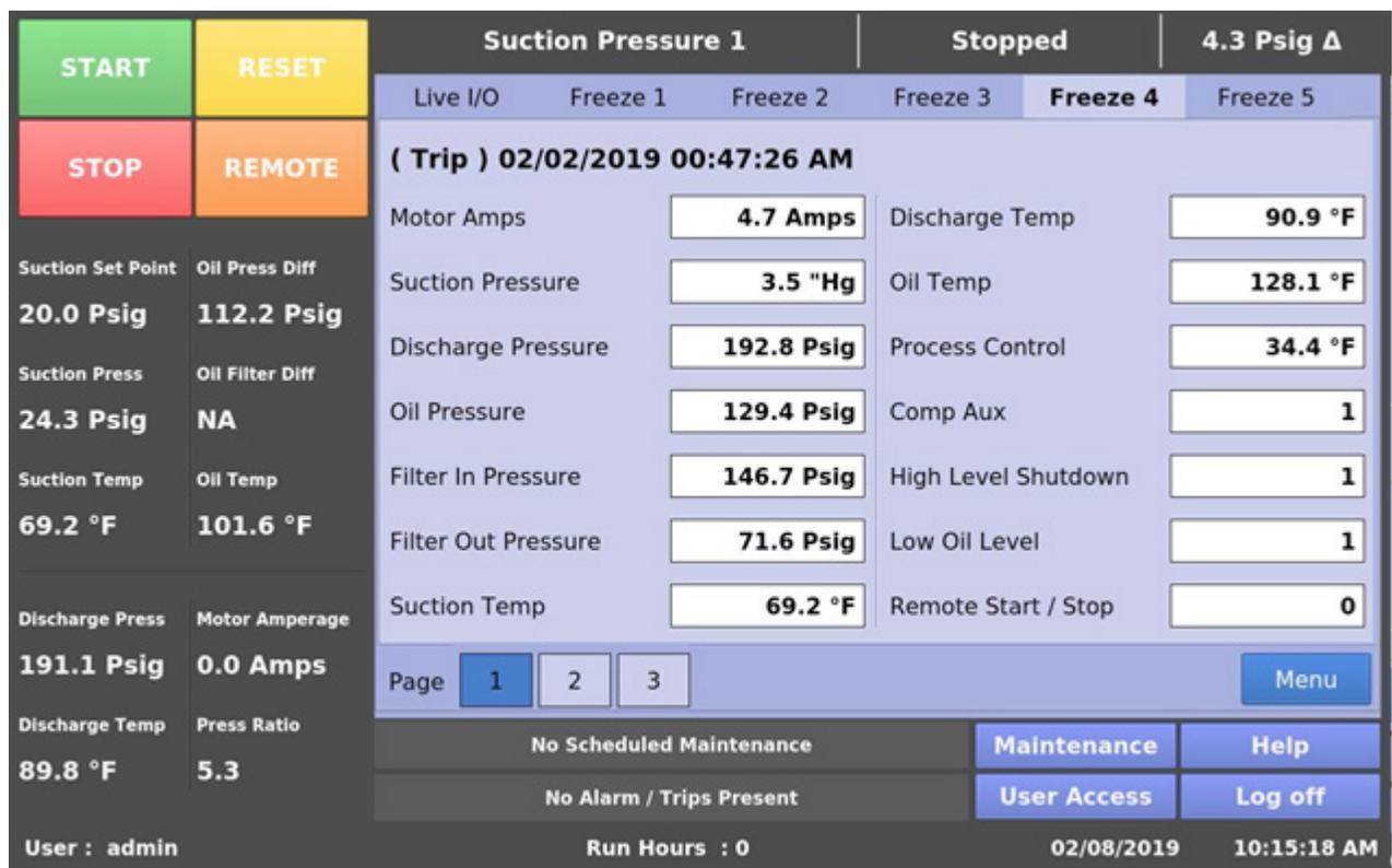
Figure 10-5. Input/Output States Screen - Freeze Data (Trip Condition)
