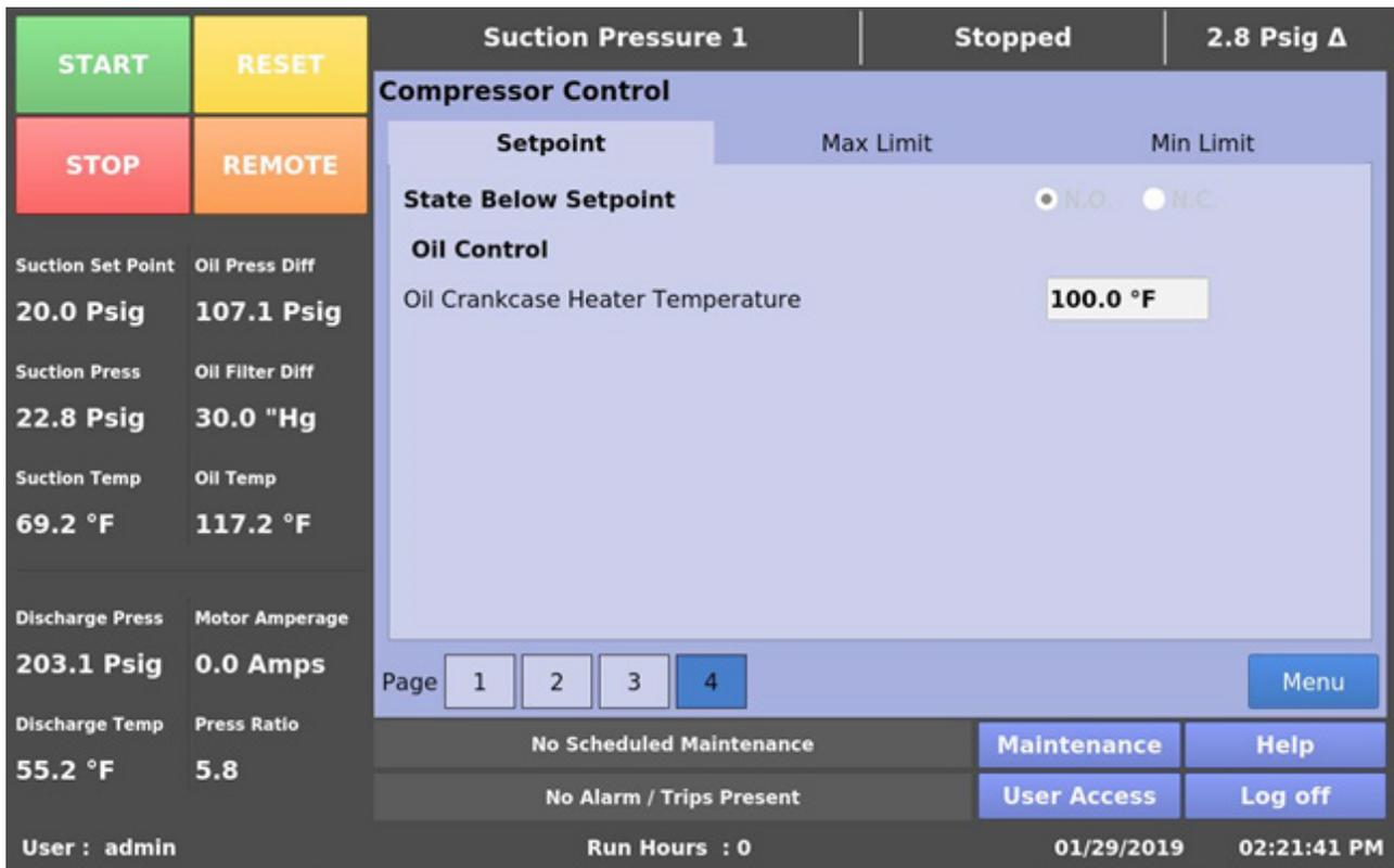
Figure 5-9. Compressor Control Screen - Oil Control
