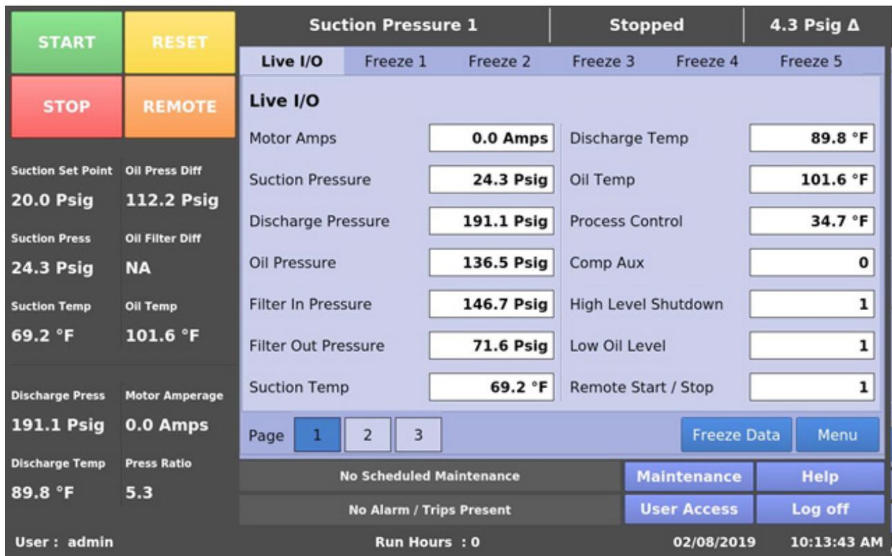
Figure 10-1. Input/Output States Screen Page 1 - Live I/O Data
