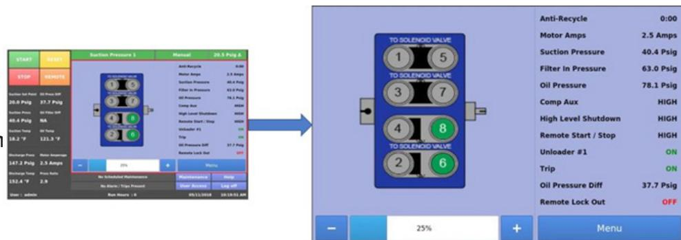
Figure 3-8. Manual Run Mode Buttons And Progress Bar
