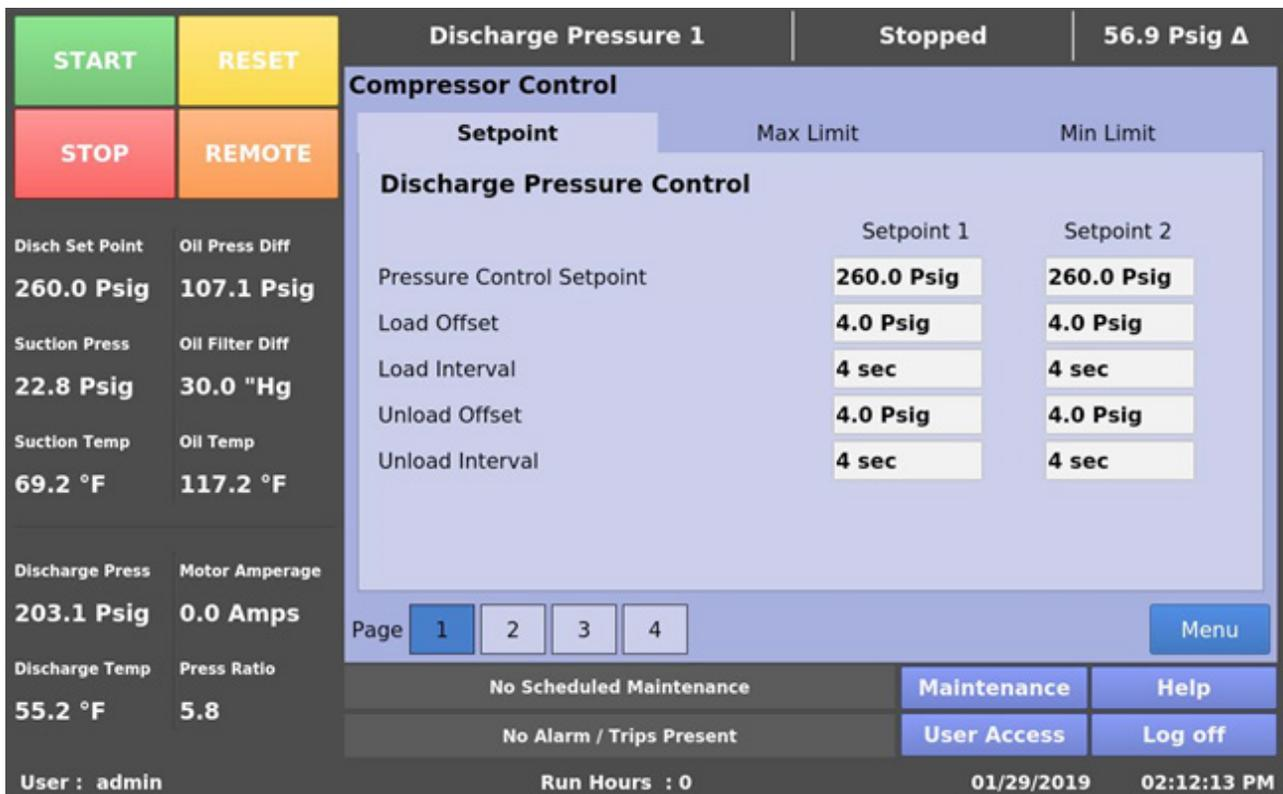
Figure 5-3. Compressor Control Screen - Discharge Pressure Control
