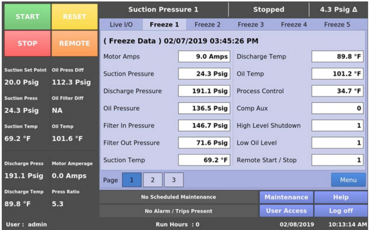
Figure 10-4. Input/Output States Screen - Freeze Data
