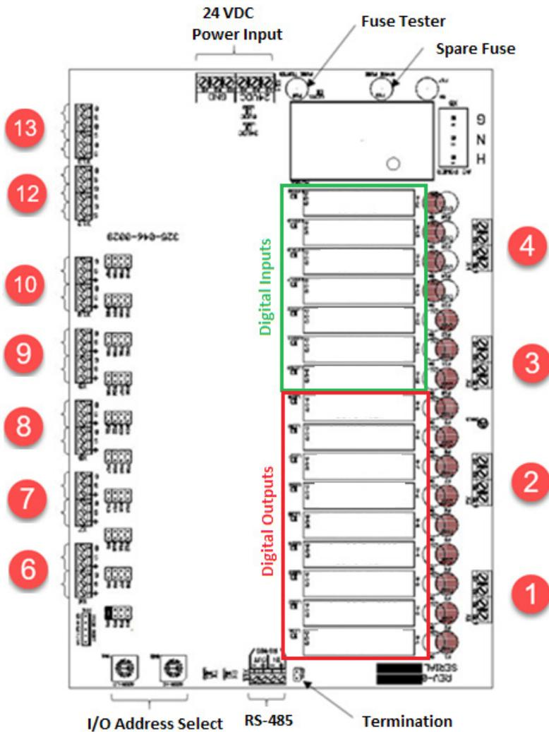
Figure 2-2. Multi I/O Board Layout
