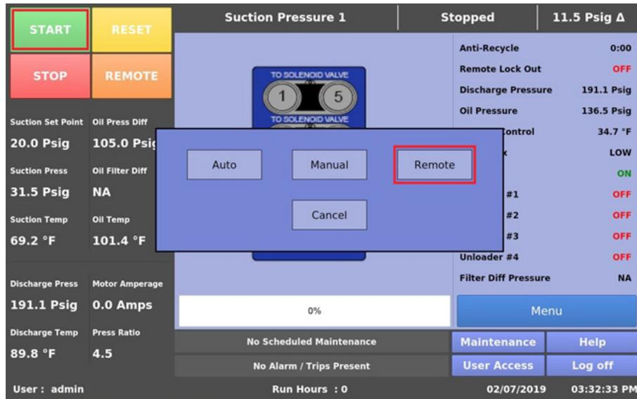
Figure C-3. Setting MicroVission in Remote Mode
