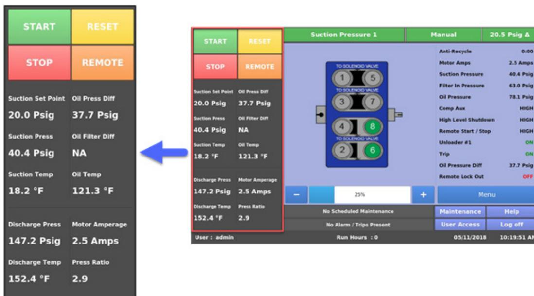
Figure 3-3. Parameters Bar
