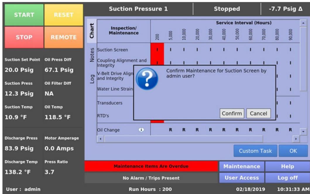
Figure 14-5. Maintenance Screen – Confirmation for Maintenance Sign-Off
