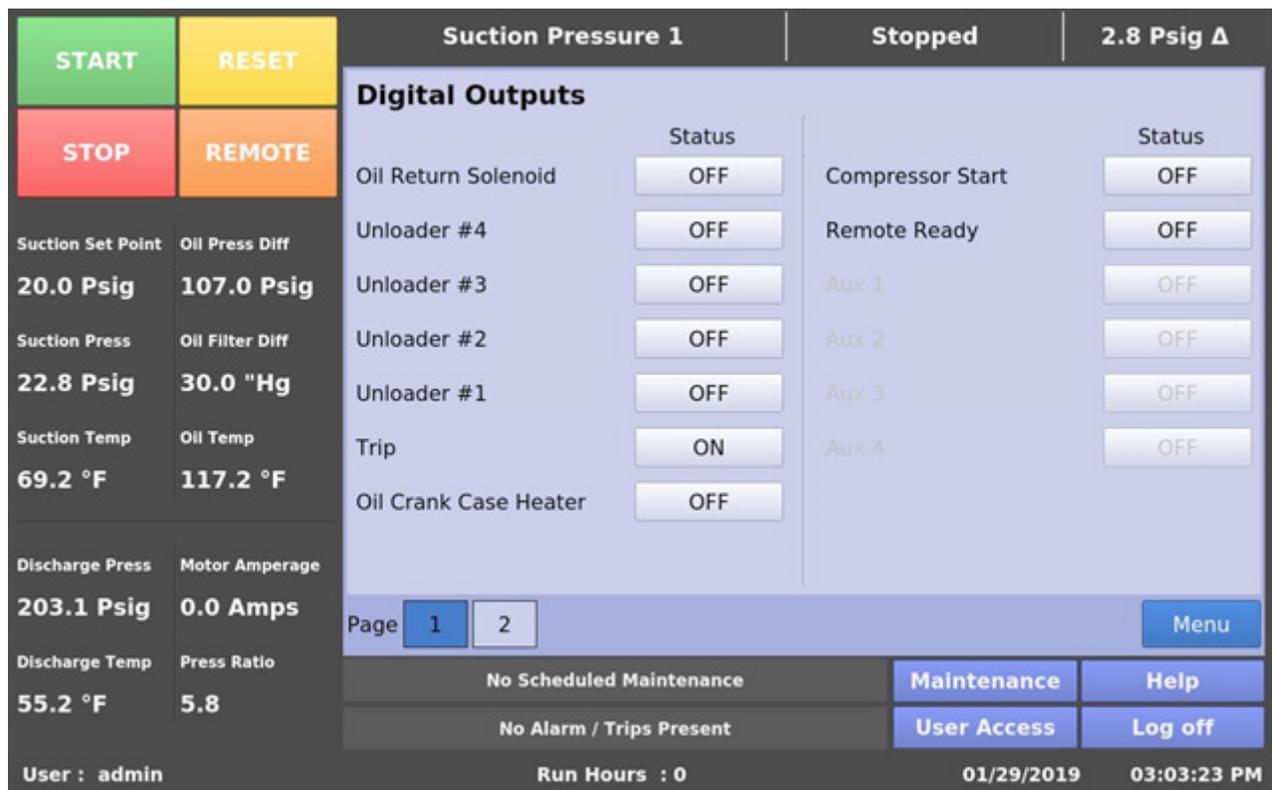
Figure 16-1. Service Options Screen Page 1 – Digital Outputs
