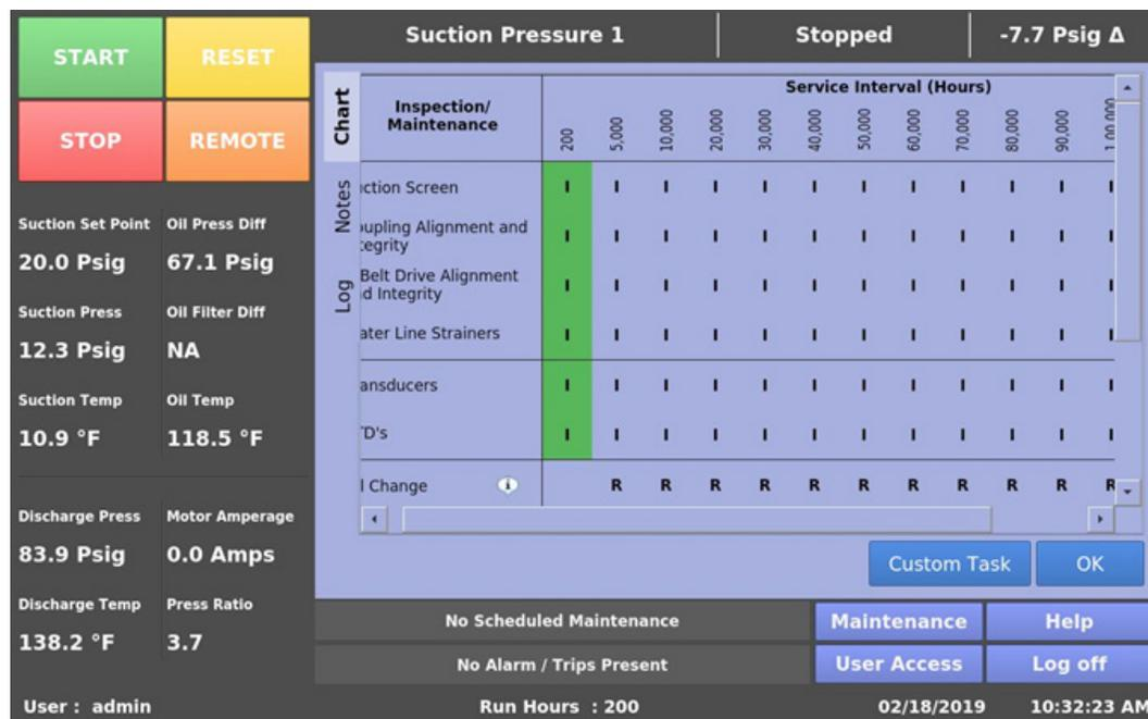
Figure 14-6. Maintenance Screen – Maintenance Sign-Off Has Been Performed
