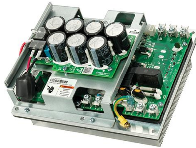
Motor Drive / Inverter
