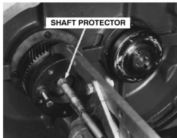
FIGURE 6-4 – BEARING PRESS PLATE
