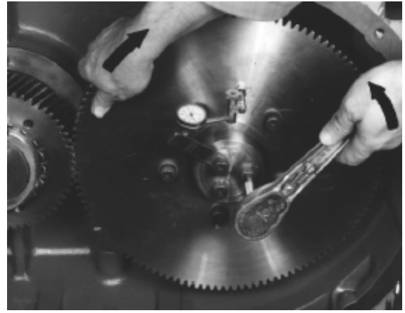
FIGURE 7-29 – SMALLEST PLUS READING
