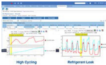
CBM alerts allow you to see error conditions such as high compressor cycling and refrigerant leaks.
