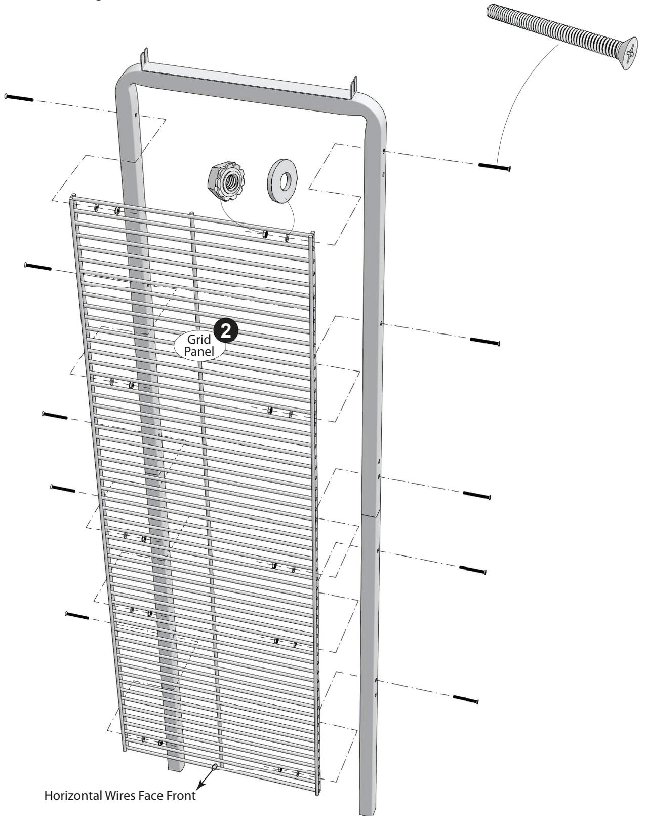
**3.** Place the tube ends of the frame assembly over the joiners of the base, then use two screws to secure.
