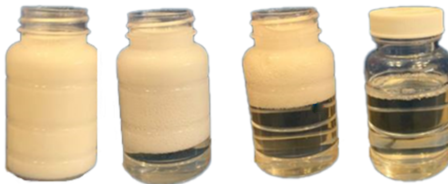
Figure 5-7. Stages of the Oil Sample Taking Process
