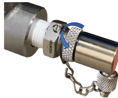
(c). Valve shown in lockout position
