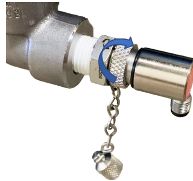
(b). Valve shown ready for oil sampling
