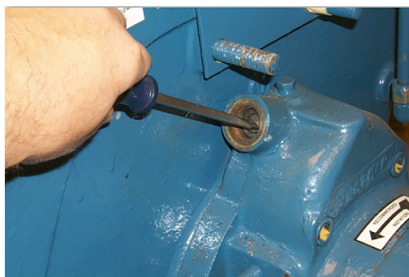
Figure 4-2. Oil Pressure Regulating Valve Adjustment
