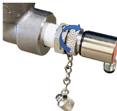
(b). Valve shown ready for oil sampling
