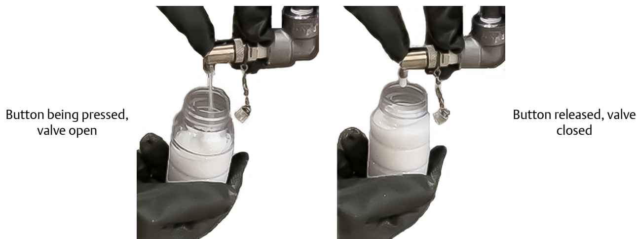
Figure 5-6. Operating the Oil Sampling Valve
