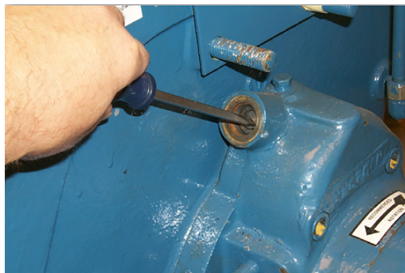
Figure 4-2. Oil Pressure Regulating Valve Adjustment
