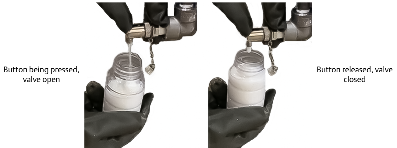
Figure 5-5. Operating the Oil Sampling Valve
