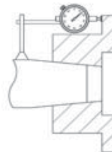
Figure 5 - Dial indicator placement for axial draw measurement example.
