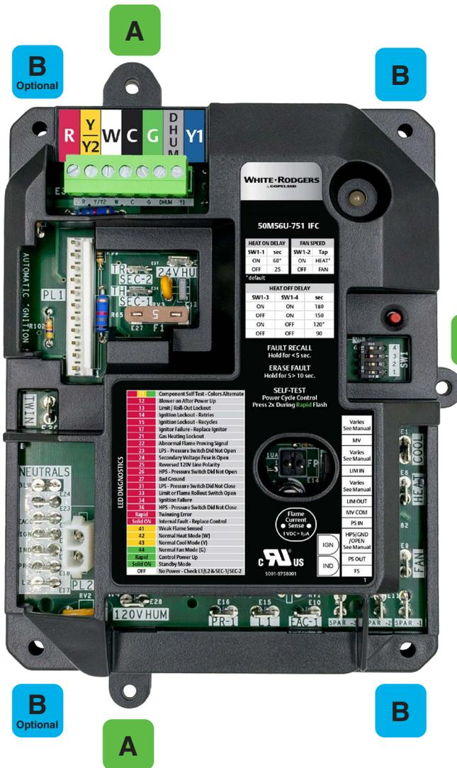
**A** **Tabs:** For OEM direct mounting when replacing controls with a **tray**. Secure with a 1/2" screw.
