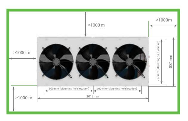
Figure 13. 20HP Unit fixing
