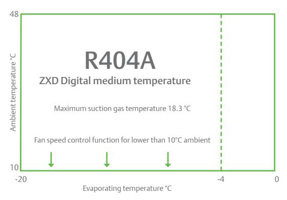
Note: ZXD120/160BE maximum evaporating temperature is 0 °C; ZXD200BE maximum evaporating temperature is -4°C
