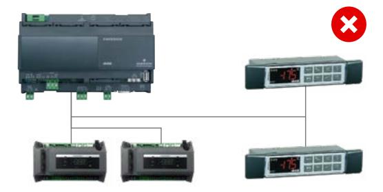
Figure 10. Incorrect network wiring
