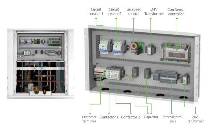
Figure 3. Electrical module of 12-16HP Large ZX
