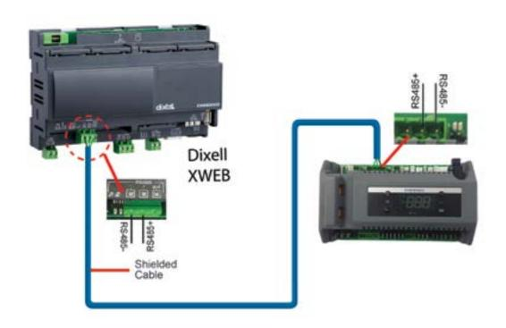
Figure 11. XWEB connected to the Intelligent Store Solution module
