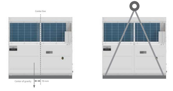
Figure 15. 20HP Unit lifting
