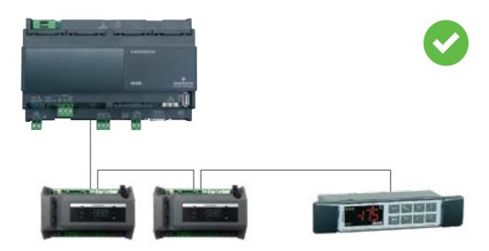
Figure 9. Correct network wiring
