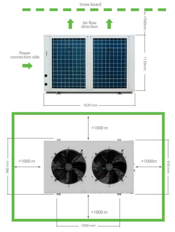
Figure 12. 12-16HP Large ZX fixing
