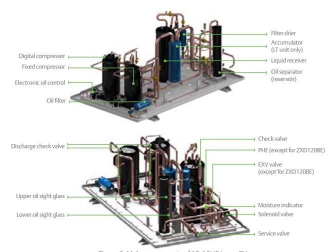
Figure 2. Main components of 12-16HP Large ZX
