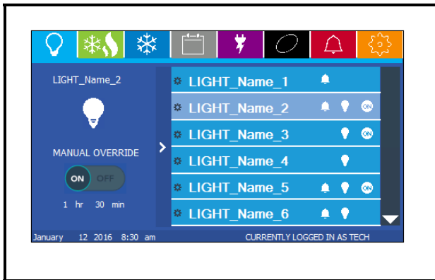
Figure 4-17 - Lighting Control Applications and Status
