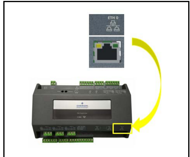
Figure 8-2 - Site Supervisor ETH0 Port
