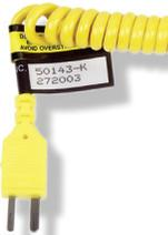
**Probes with Cables** – The serial number is located on the label fastened just above the mini-connector.
