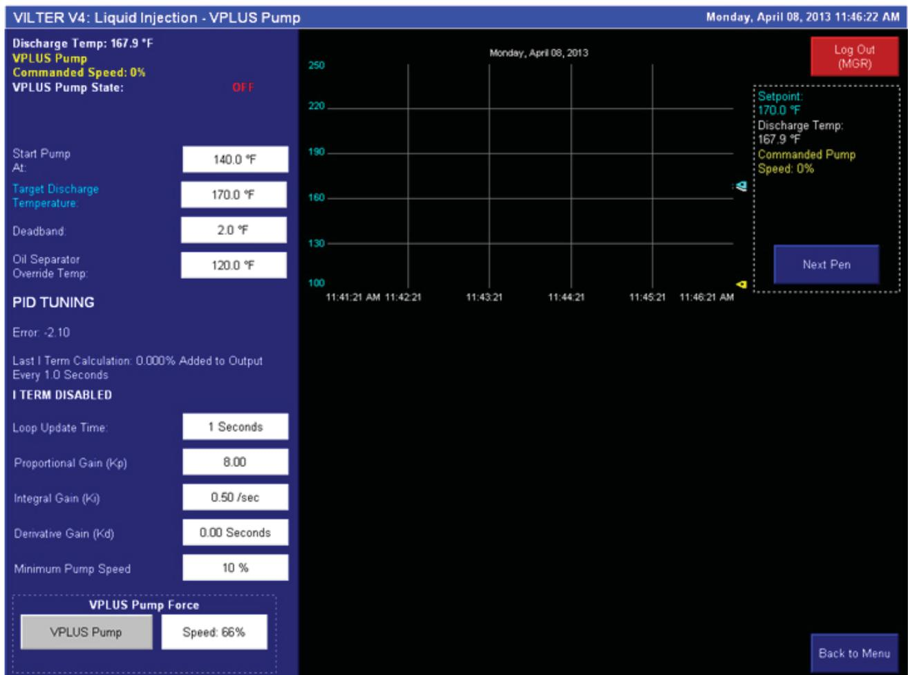
Figure 9-11. Liquid Injection (VPLUS Pump) Screen
