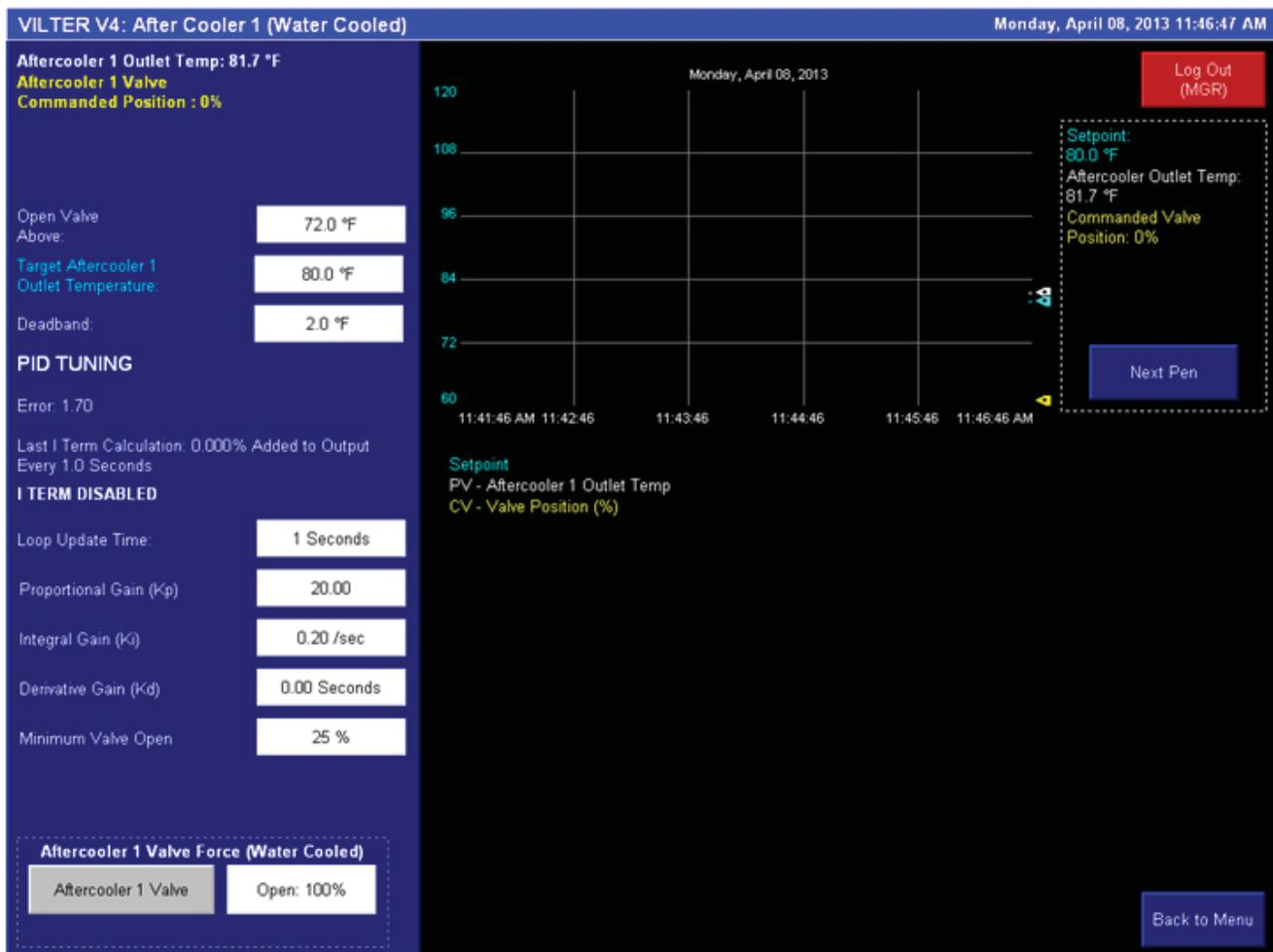
Figure 9-6. Water Cooled Aftercooler Screen
