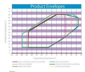
Notes: Dashed Red Line 1 Indicates 63 °C Condensing Limit For ZP51 To ZP61K5E - PFV For -5% Voltage Tolerance Dashed Red Line 2 Indicates The Limit Of Operation With Constant Return Gas Temperature of 35 °C \*Does Not Include ZP91, ZP104, ZP122KCE
