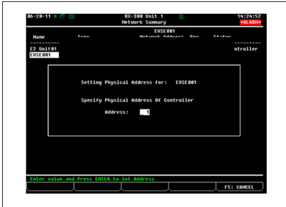
Figure 14 - Device Physical Address Setting
