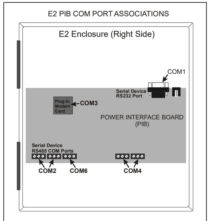
Figure 16-3 - Location of E2 COM Ports - E2 PIB Board (E2 version 4.2 and above)
