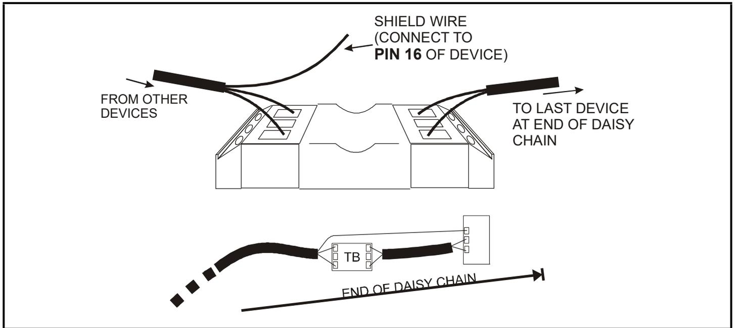
Figure 16-9 - MODBUS Termination Block (P/N 535-2711)
