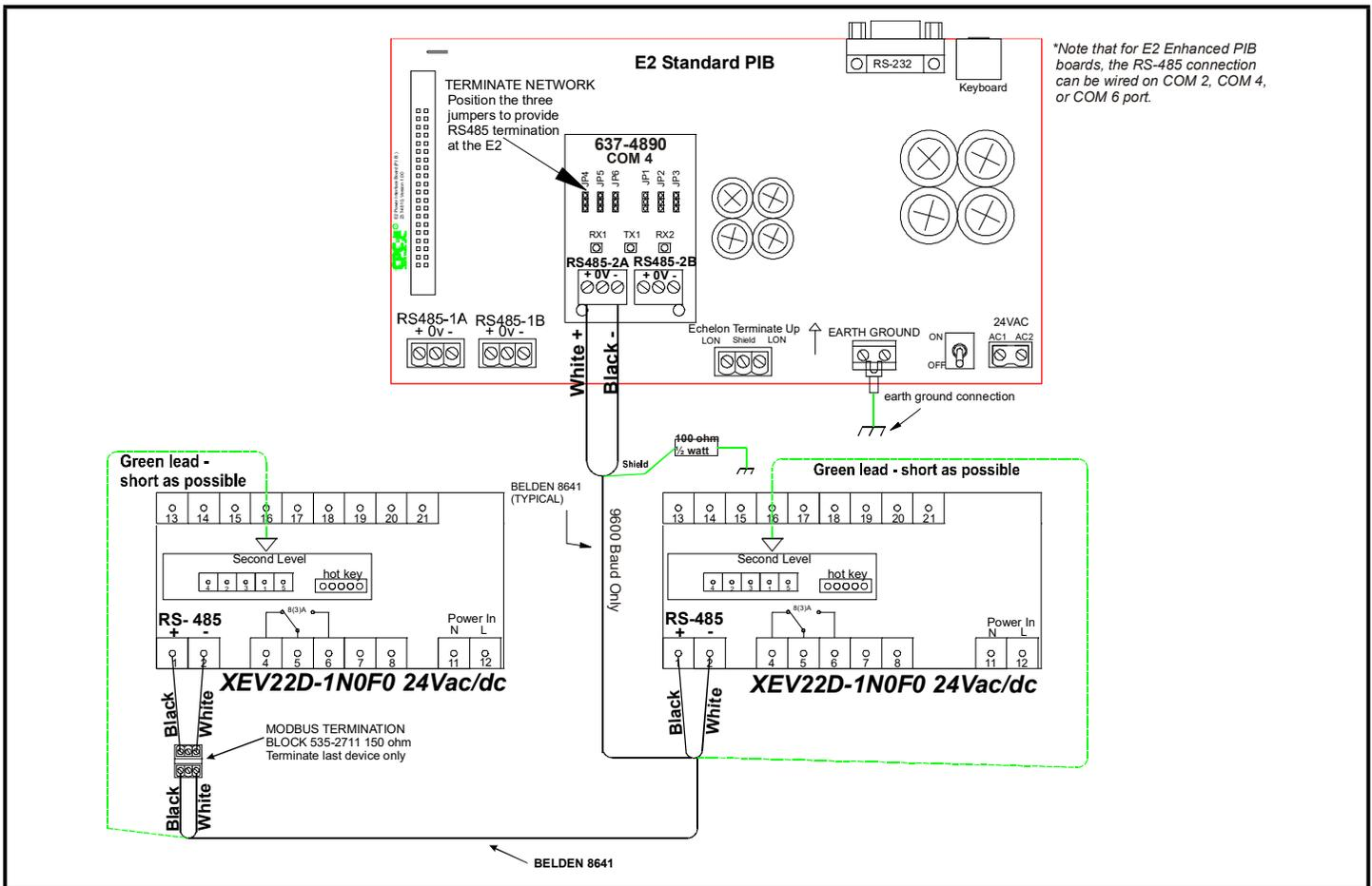
Figure 15-1 - XEV22D to E2 Wiring Diagram (E2 PIB version 3.xx and below shown in this example)
