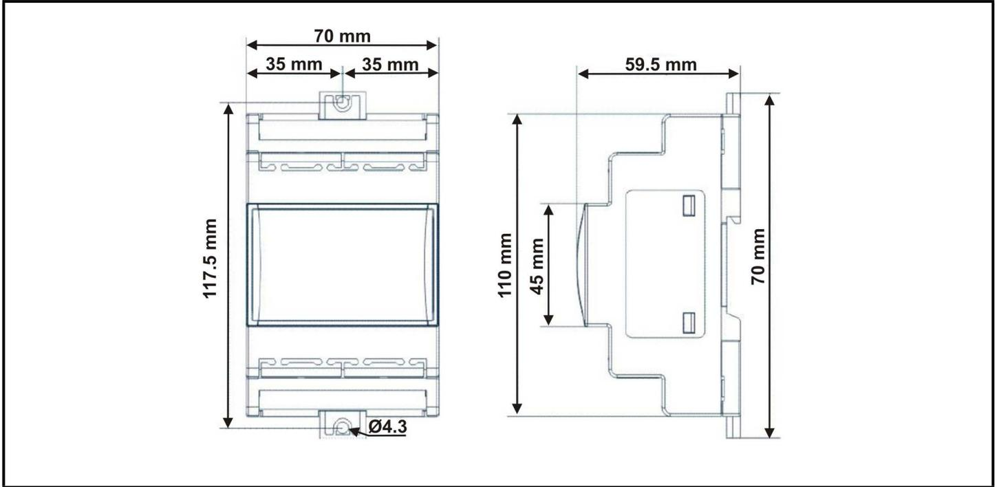
Figure 5-1 - DIN Mounting
