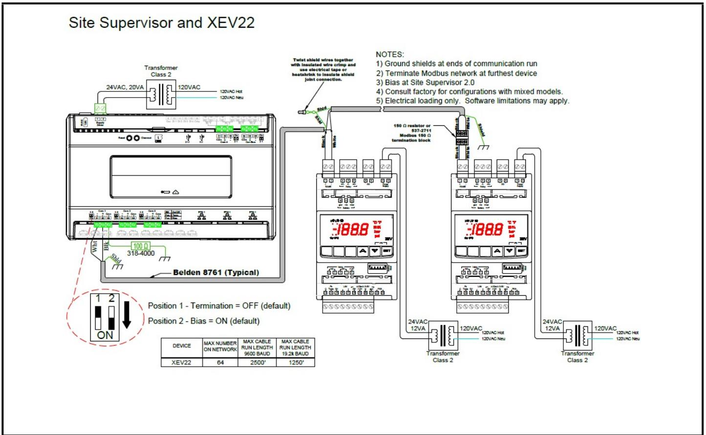
Figure 5-2 - Site Supervisor Wiring
