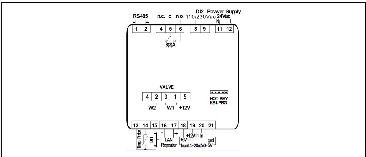
Figure 4-2 - XEV22D Wiring Connections
