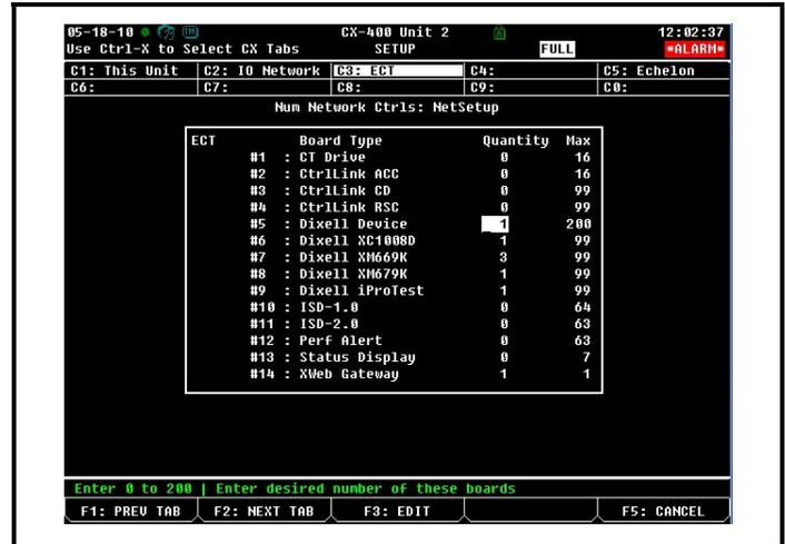
Figure 16-5 - Num NetworkCtrls: NetSetup Screen
