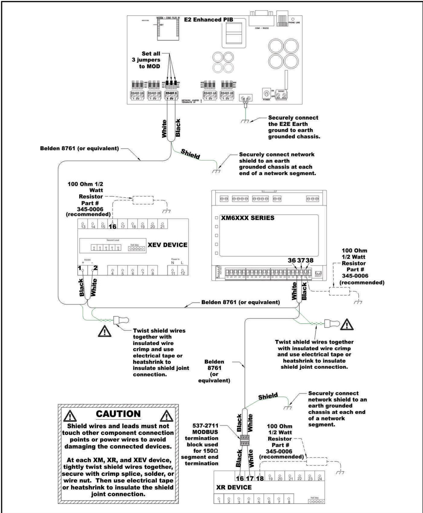
Figure A -1 - MODBUS Com Wiring Diagram
