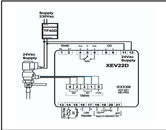
Figure 4-8 - Transformer Connection (24VAC Coil)
