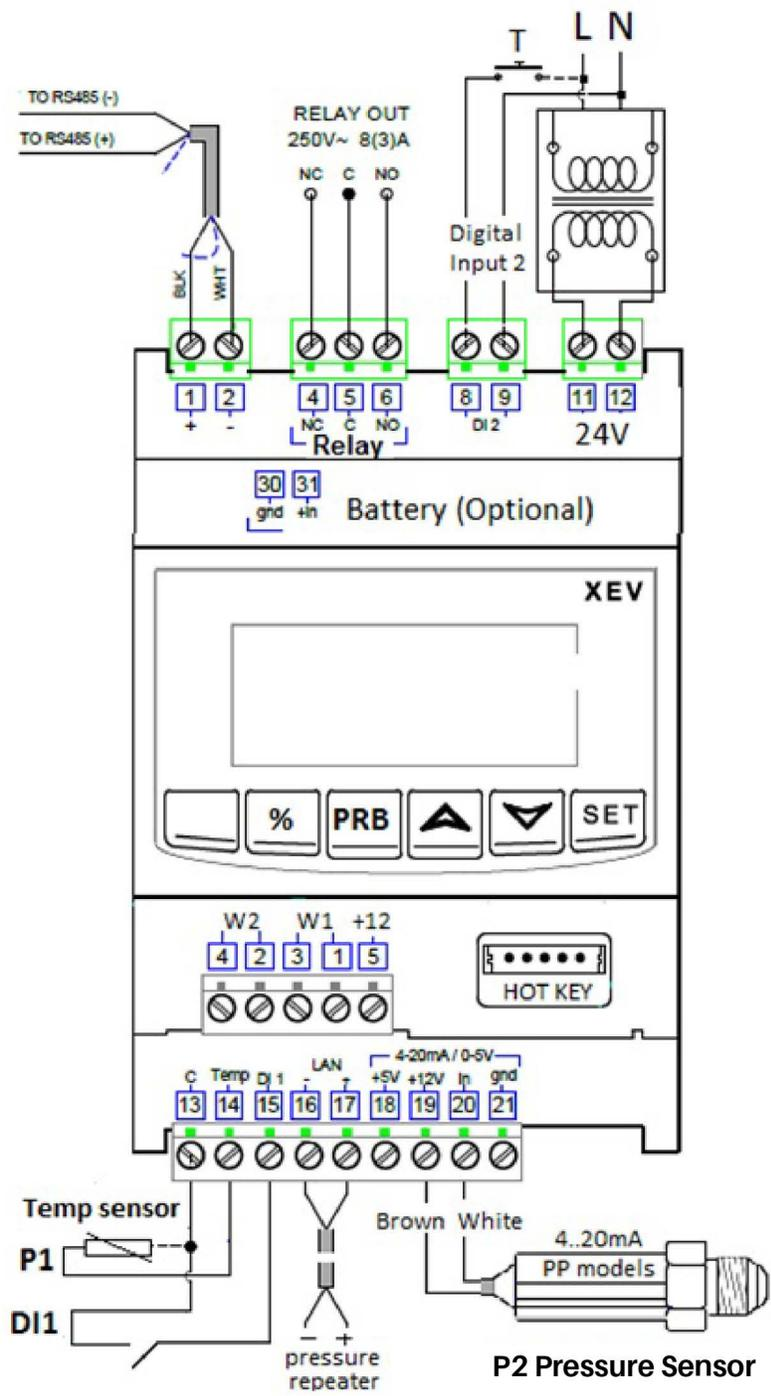
Figure 4-3 - XEV22D Release 1.5 Wiring Connections
