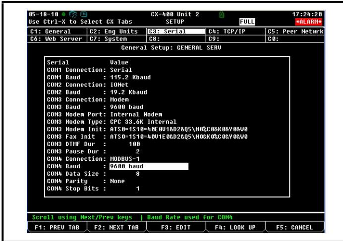
Figure 16-4 - Serial Communications Manager Screen
