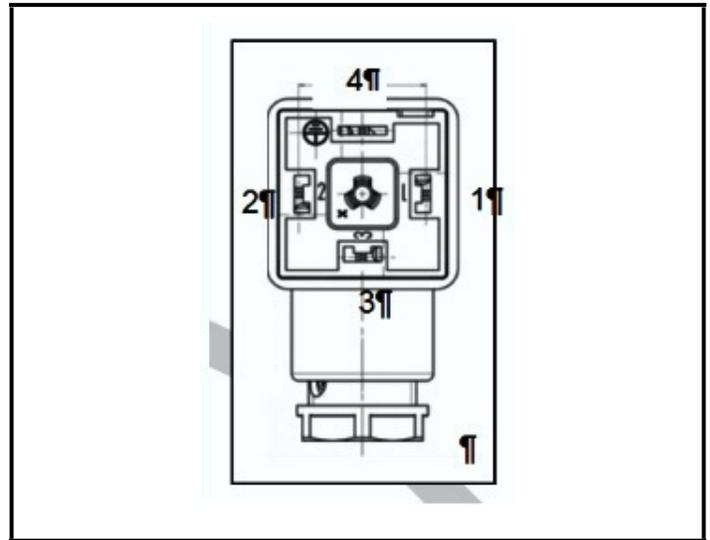
Figure 4-6 - Solenoid Valve Connection
