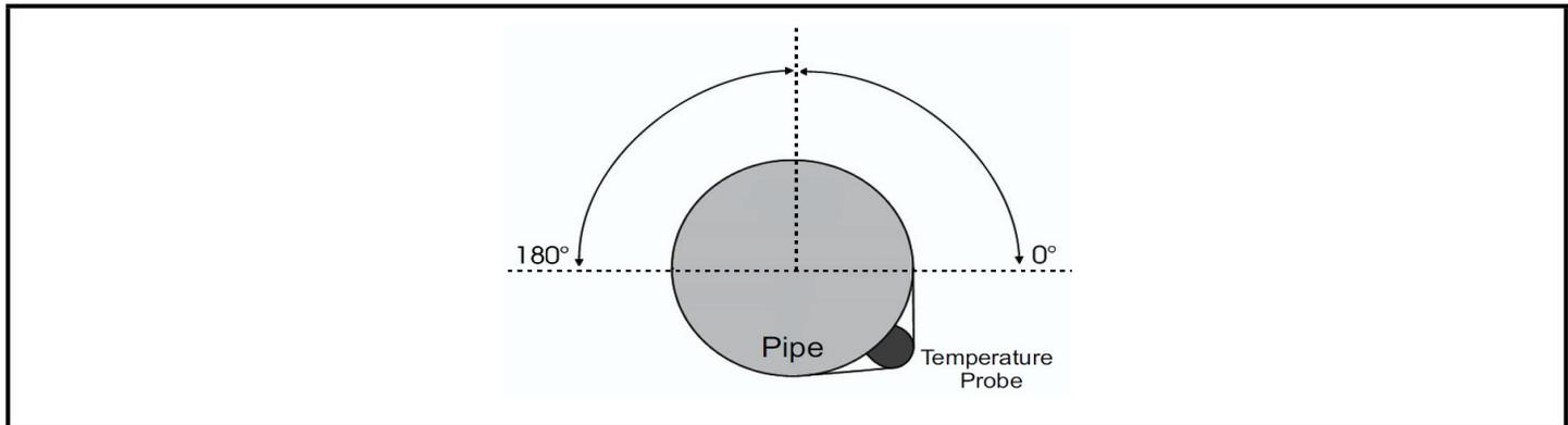
Figure 4-4 - Temperature Probe Placement
