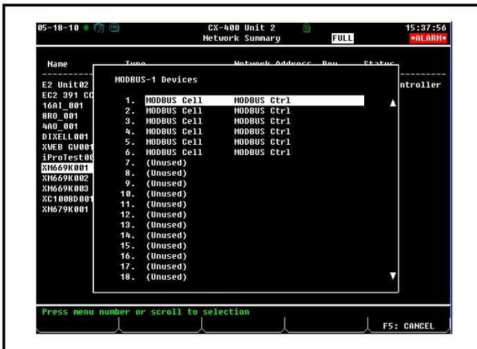
Figure 16-7 - List of MODBUS Devices
