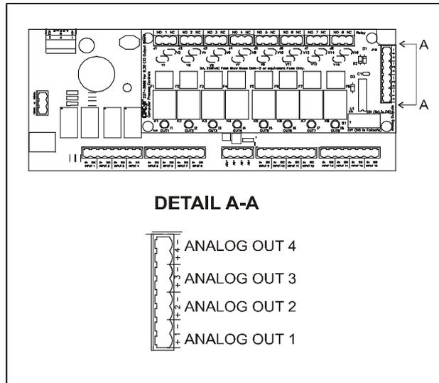
Figure 4-7 - MultiFlex RCB Analog Output Locations
