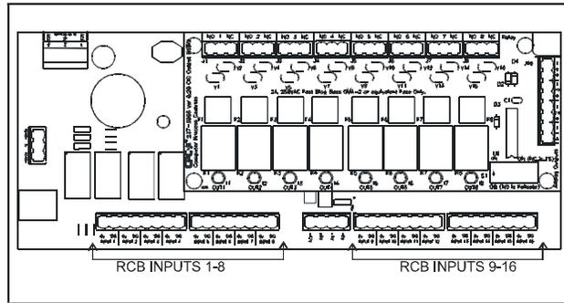
Figure 4-1 - MultiFlex RCB Input Locations
