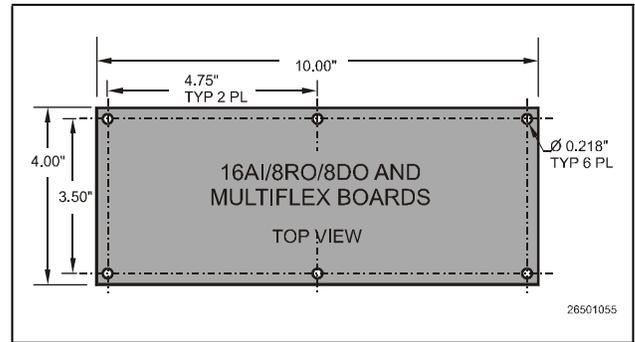
Figure 2-2 - MultiFlex Board Dimensions
