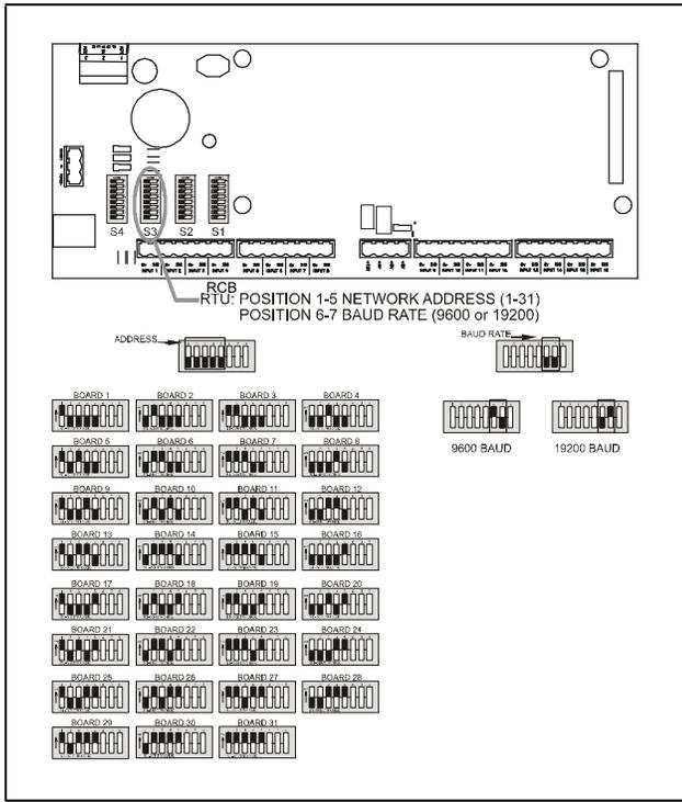
Figure 3-2 - RCB Baud Rate Switches
