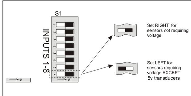
Figure 4-3 - Input Type Dip Switches for RCB Board
