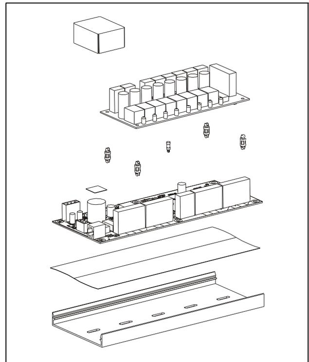
Figure 2-3 - Exploded View — MultiFlex RCB
