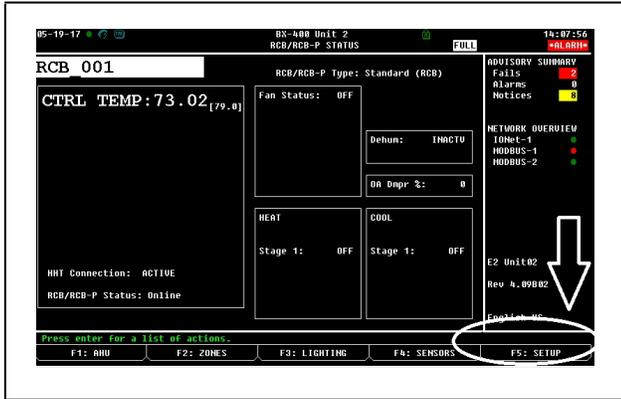
Figure 7-6 - RCB Status Screen - Press F5 for Setup
