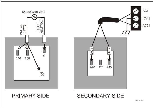
Figure 2-4 - Wiring Non-Center Tapped MultiFlex Boards to Transformers With a Center Tap
