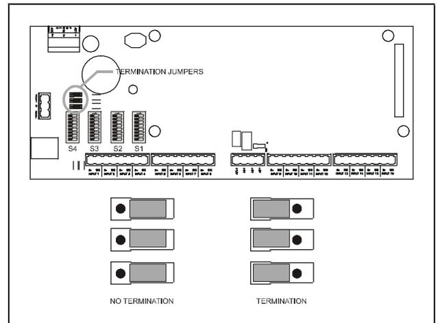
Figure 3-3 - I/O Network Termination Jumper Settings
