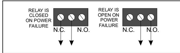
Figure 4-6 - Form C Contact Wiring
