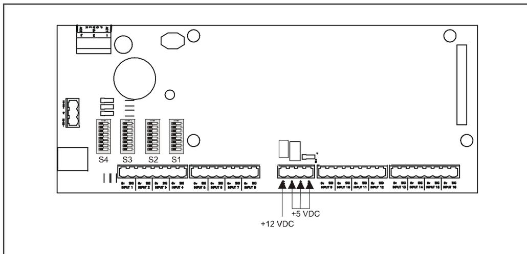
Figure 4-4 - Input Board Power Sources
