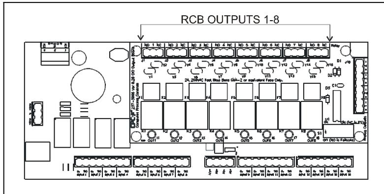
Figure 4-5 - MultiFlex RCB Output Locations
