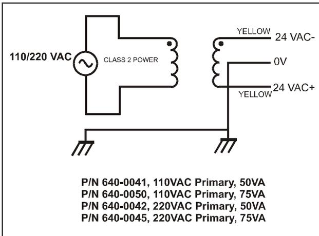
Figure 2-5 - Non-Center-Tapped Transformer Wiring
