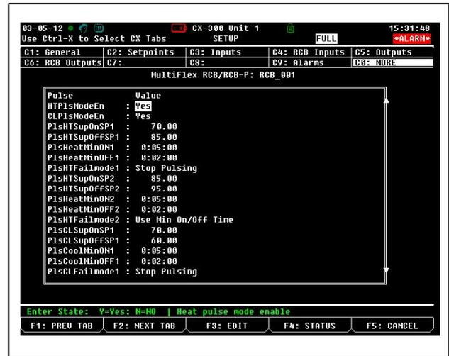
Figure 7-9 - RCB-P Pulse Control Setup Screen
