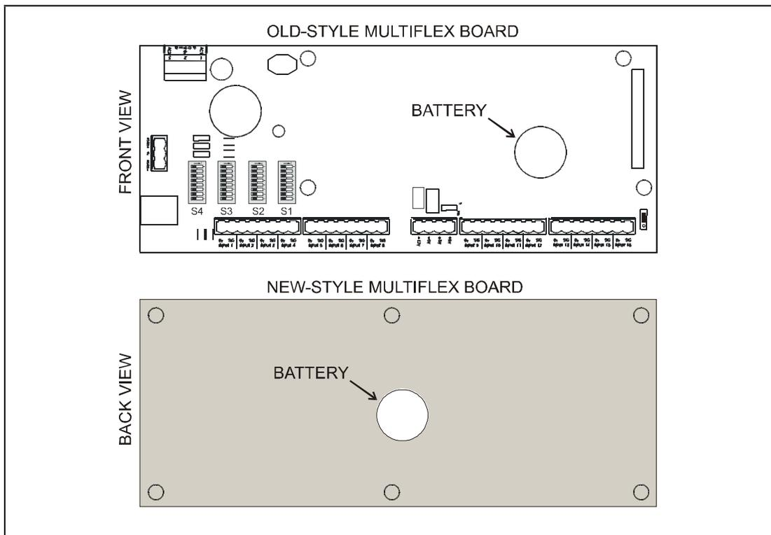
Figure 2-6 - MultiFlex Battery Location
