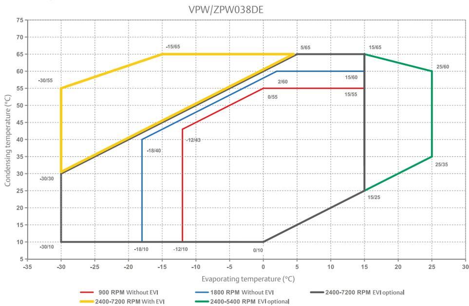
EVI technology significantly improves the operating range of compressors at low temperatures
