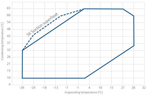
Based on: 11.1K SH, 8.3K SC, 35.0 C Ambient (Solid line boundaries) Refer to application engineering bulletin for details on the speed range throughout the operating envelope.
