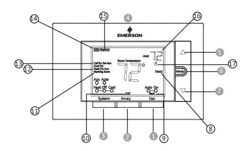
Whenever "I Replace" appears in the display, new premium brand AA alkaline batteries should be installed. If the house will be unoccupied for an extended period and either "III" or "I Replace" is displayed, install new batteries before leaving.
