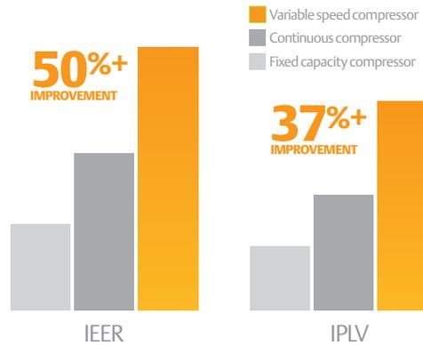
**1,000-7,200 RPM speed range for 20-100% coverage**
