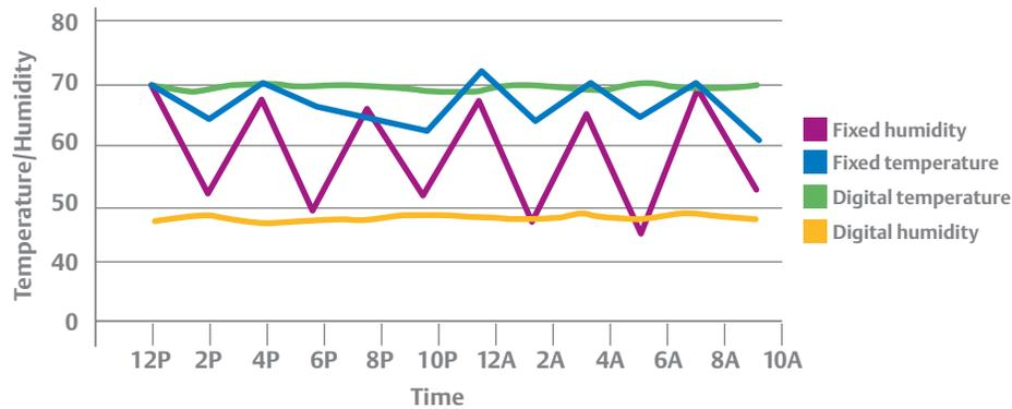
Systems with digital scroll technology are able to maintain tighter temperatures and humidity levels over fixed capacity compressors.
