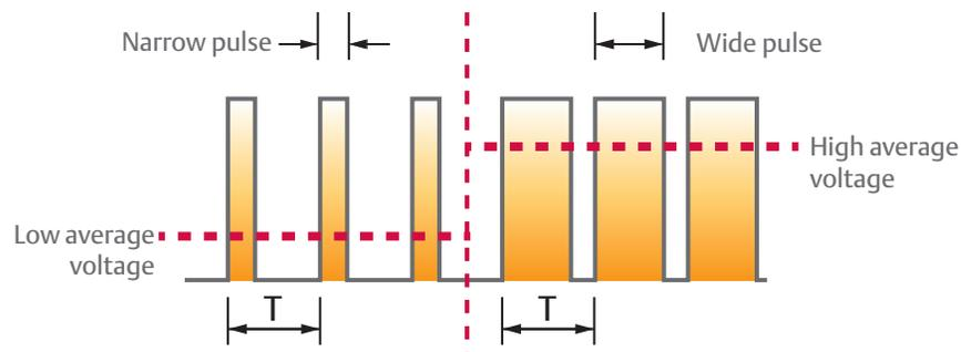
Modulation is achieved with a cycle time based on Pulse Width Modulation (PWM) control of a solenoid valve that operates a piston fitted rigidly to the upper scroll. The compressor capacity is controlled by modulating the solenoid valve input over time (T).
