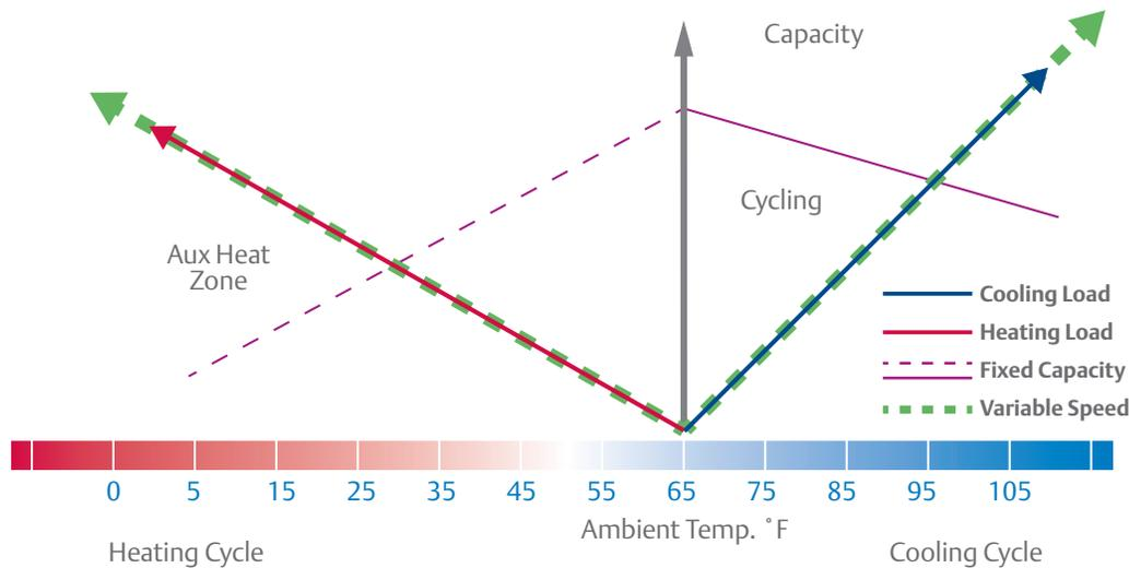
With less cycling and longer run times, variable speed compressors are able to maintain precise temperature control (roughly within 1/10th of a degree).
