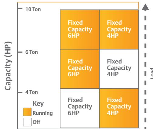
Uneven tandems can deliver three capacity stages to match the loads as the demand increases
