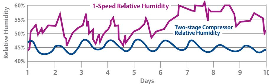
Field testing shows improved temperature and humidity control provided by Copeland Scroll two-stage compressors compared to fixed compressors.
