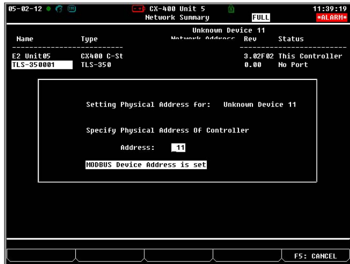
Figure 8 - MODBUS Physical Address Commissioned
