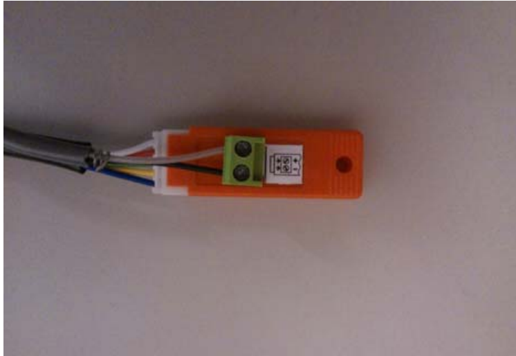
Figure 8 - Device Wiring Using TTL/RS485 Serial Converter
