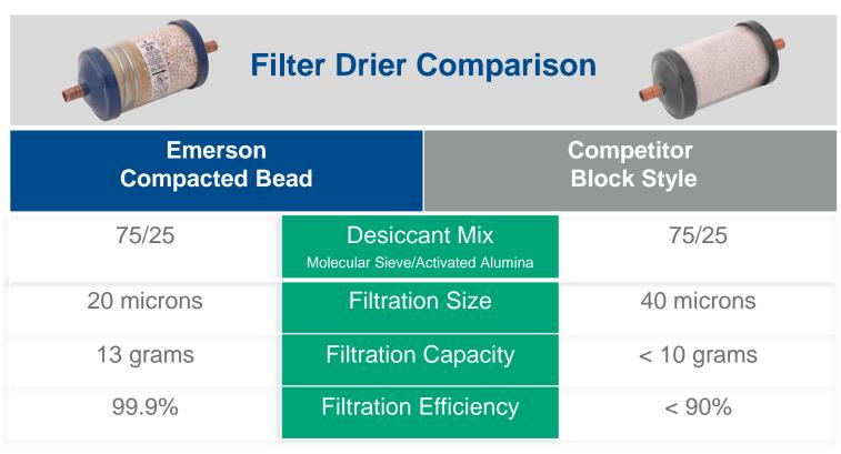
Calculations based on 16 cu. in. drier
