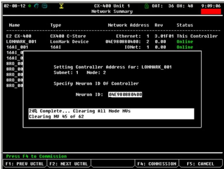
Figure 9 - Identifying the controller using the neuron ID
