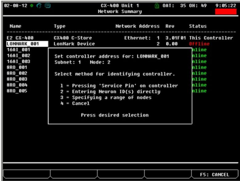
Figure 8 - select method for Identifying the controller
