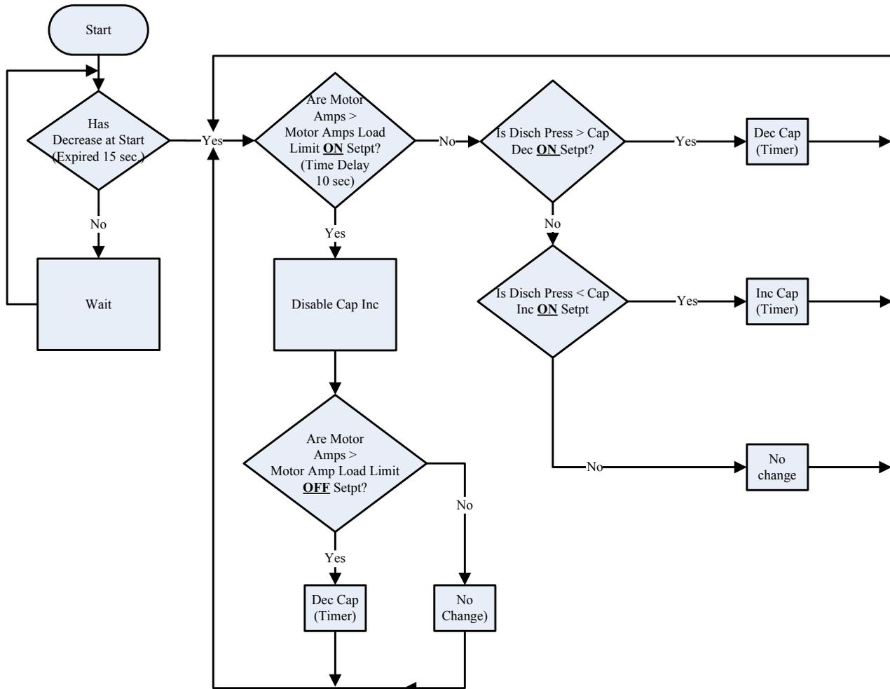
**Compressor Operation with VFD Drive**
