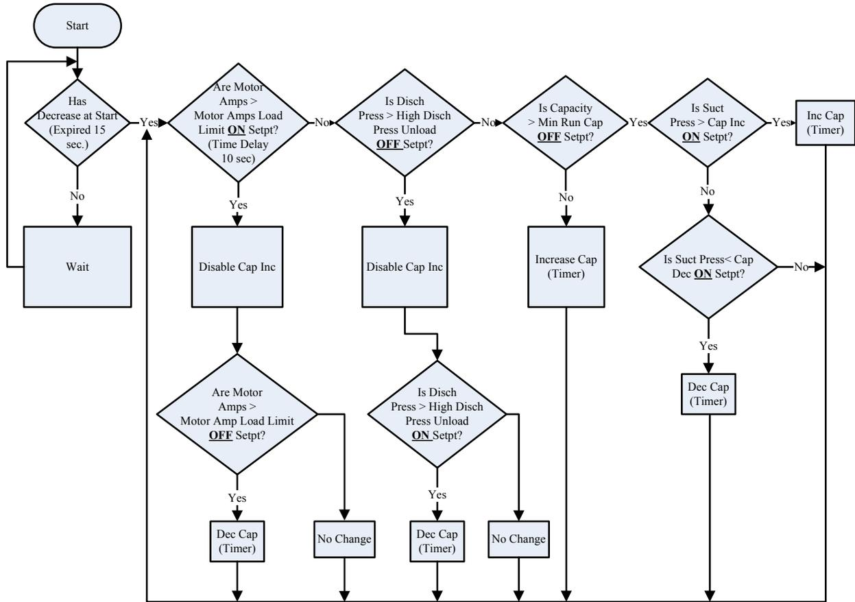
Capacity Control Using Discharge Pressure Control Setpoints
