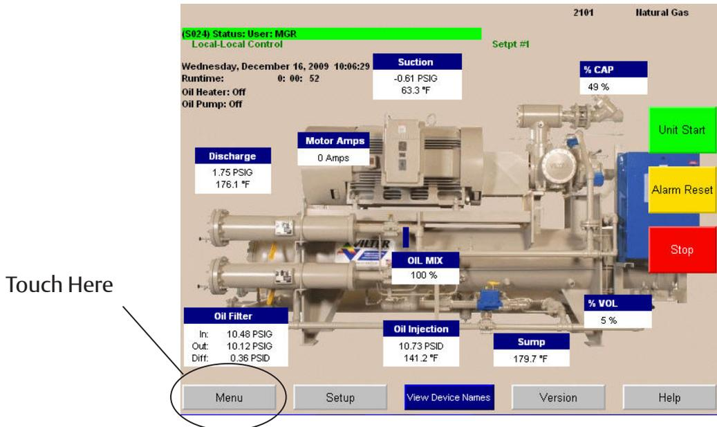
At the bottom of the **Main** screen touch the Menu button to bring up the screen shown in Figures below.
