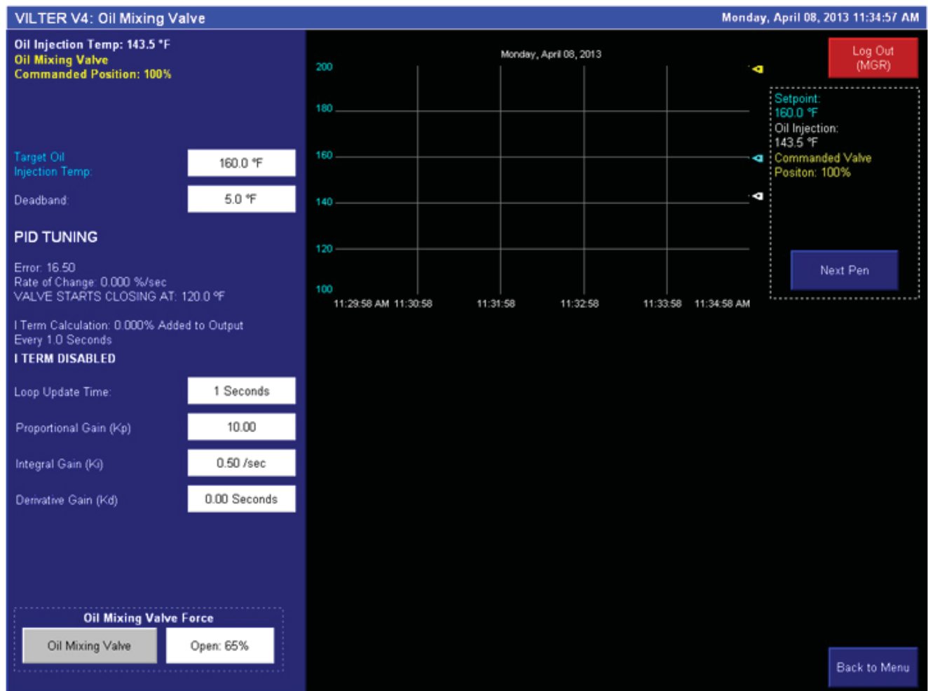
Figure 9-1. Oil Mixing Valve Screen
