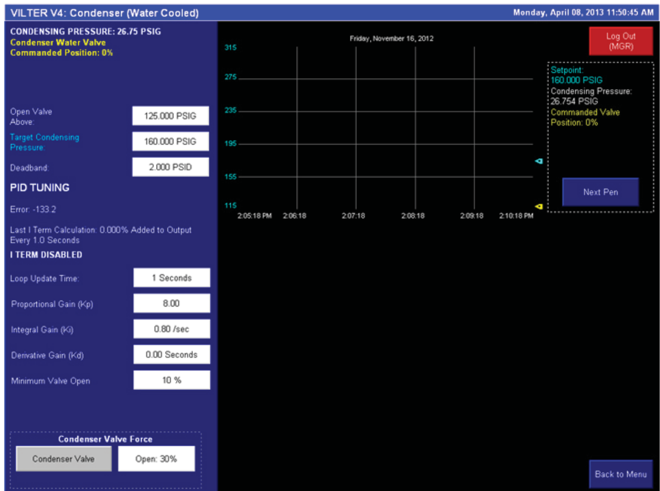
Figure 9-9. Water Cooled Condenser Screen
