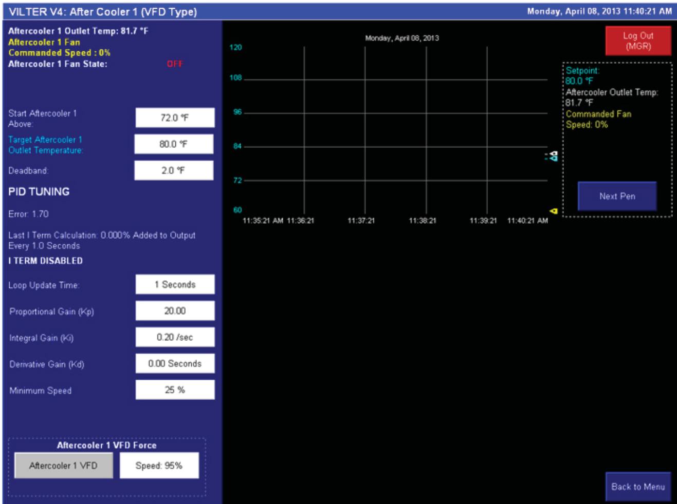
Figure 9-4. Aftercooler (VFD Type) Screen
