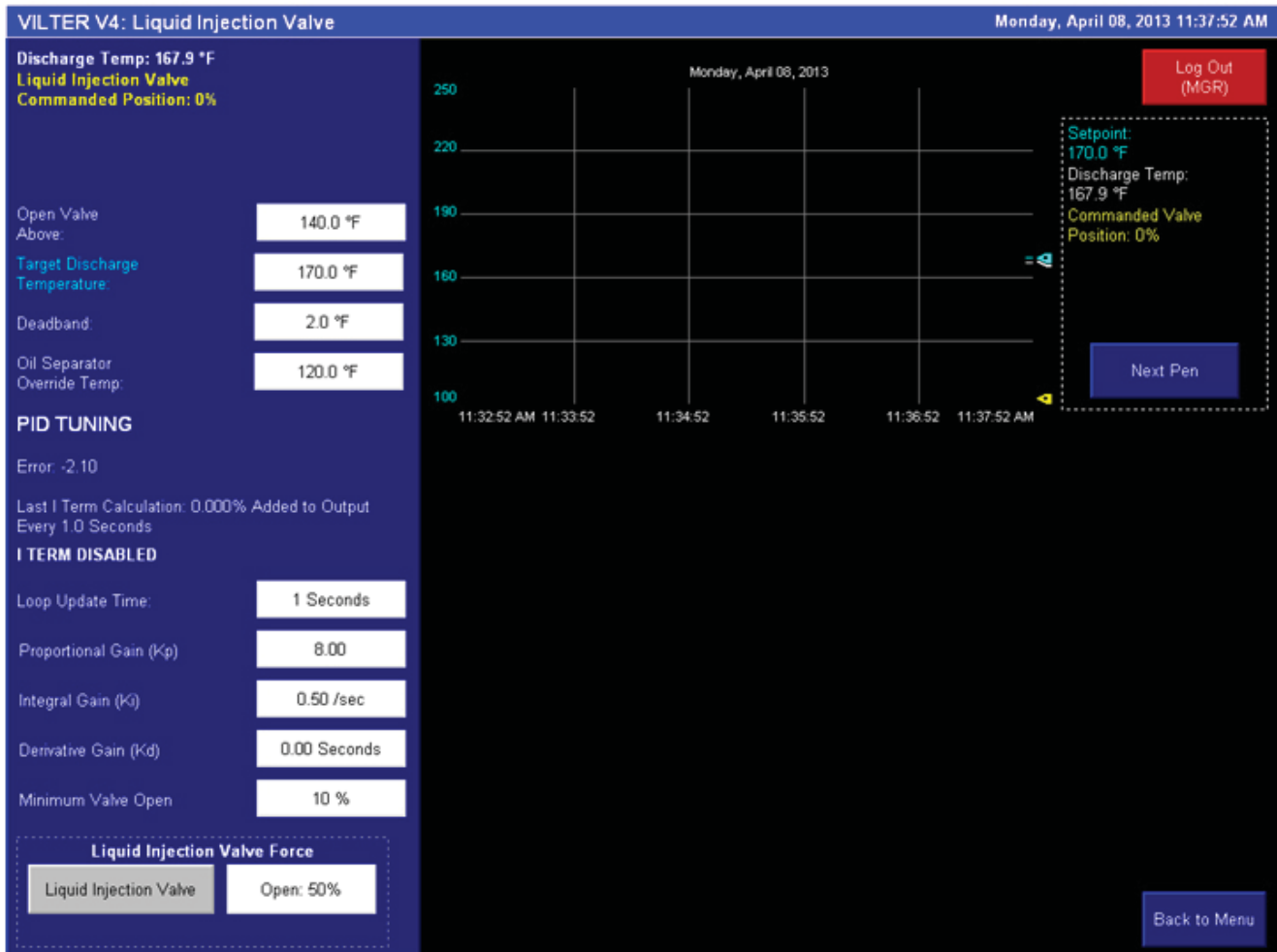
Figure 9-10. Liquid Injection Valve Screen
