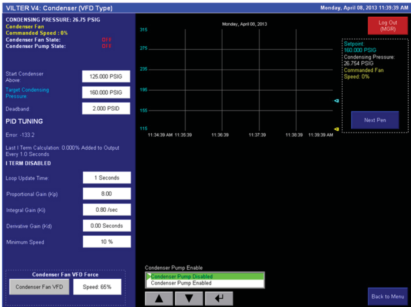
Figure 9-8. Condenser (VFD Type) Screen
