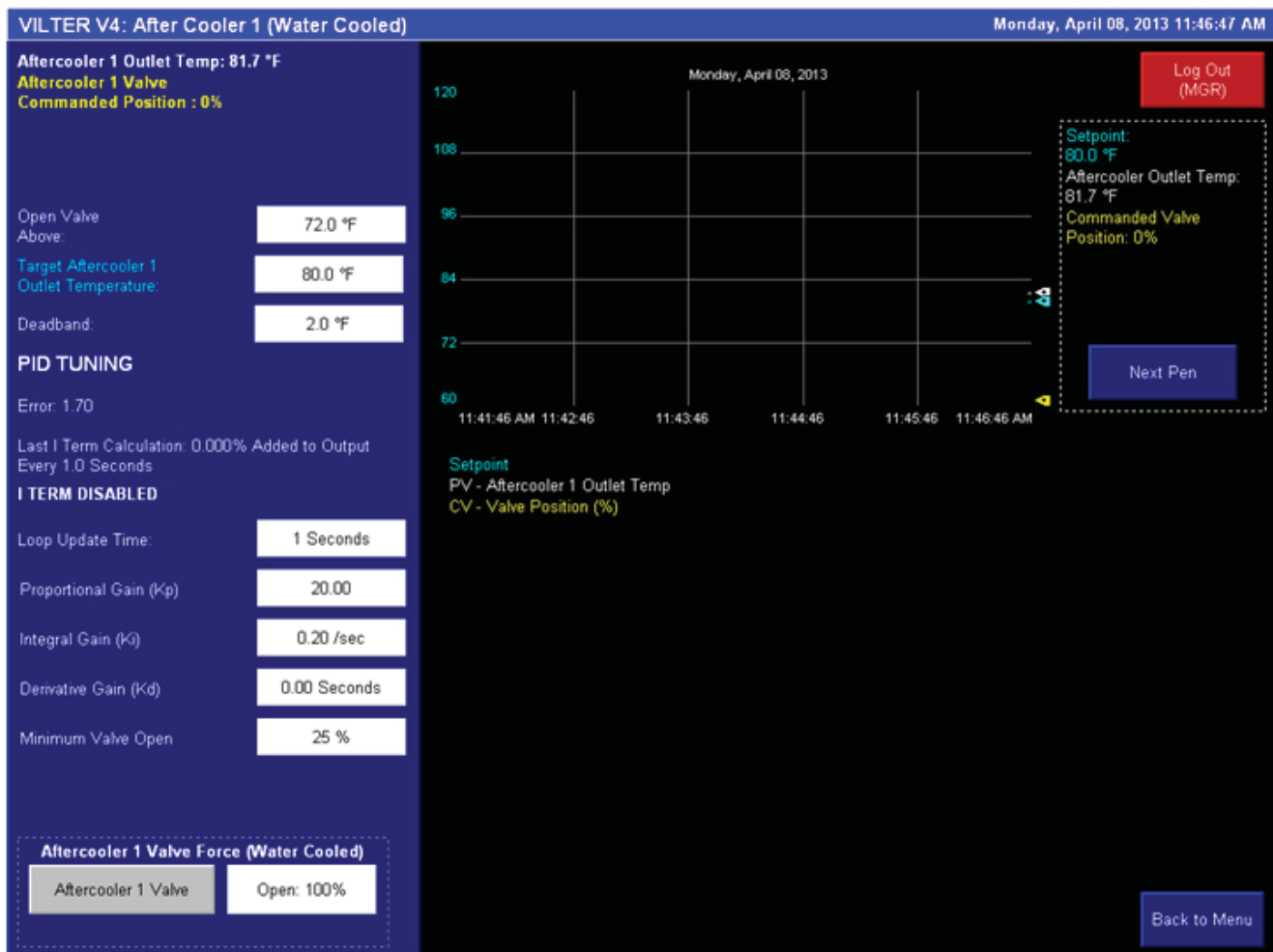
Figure 9-6. Water Cooled Aftercooler Screen
