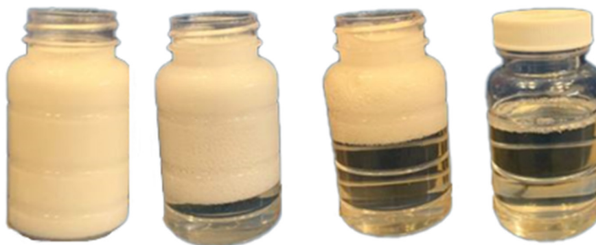
Figure 5-6. Stages of the Oil Sample Taking Process
