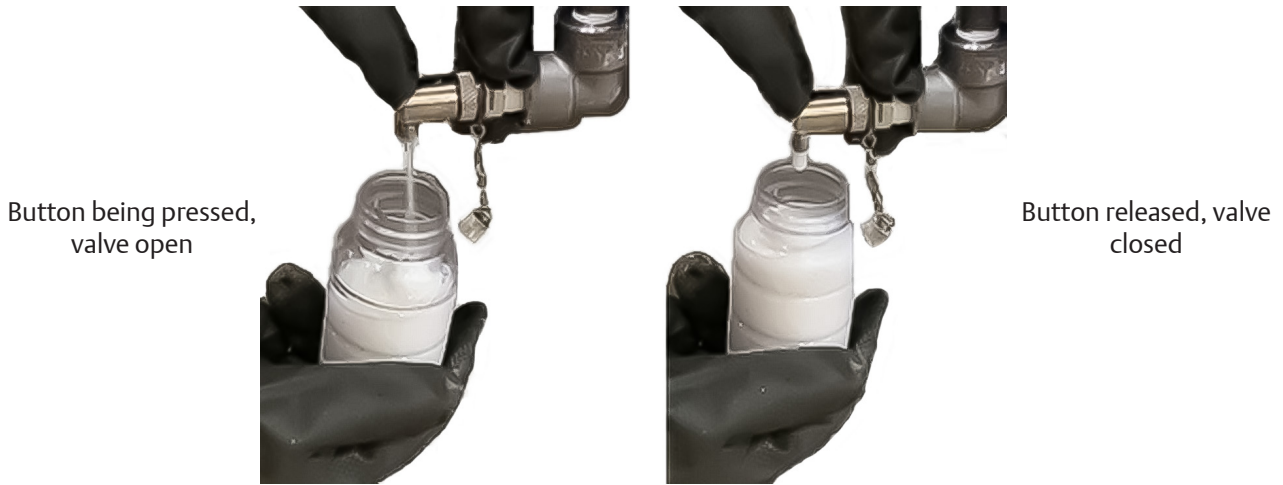
Figure 5-5. Operating the Oil Sampling Valve
