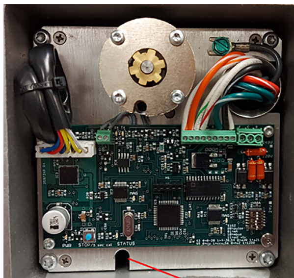
Figure 4-5. Rotation Check. Motor/Brake Shaft Spins Opposite of the Command Shaft
