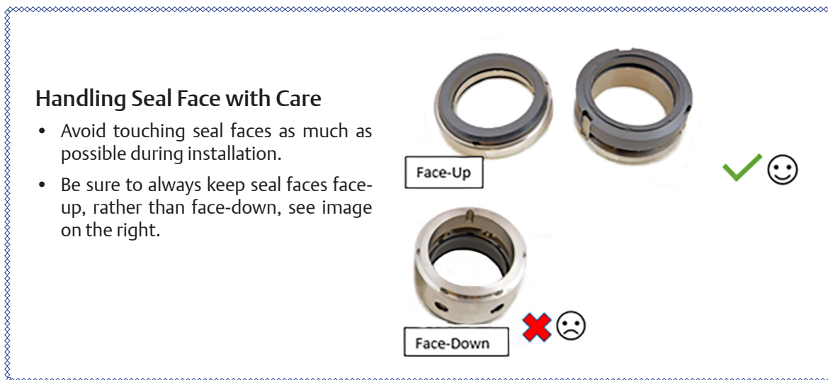
Figure 5-64. Handling Seal Face with Care
