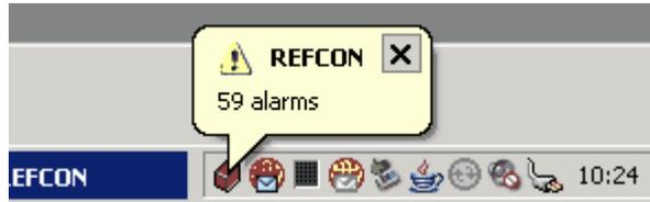
The idea of the *notify icon* is that you can use the PC for other purposes, the *REFCON Monitor* being not visible, and still be notified in case of alarms.
