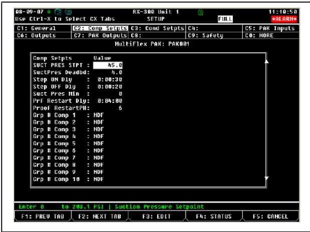
Figure 7-5 - PAK Screen 2: Compressor Setpoints
