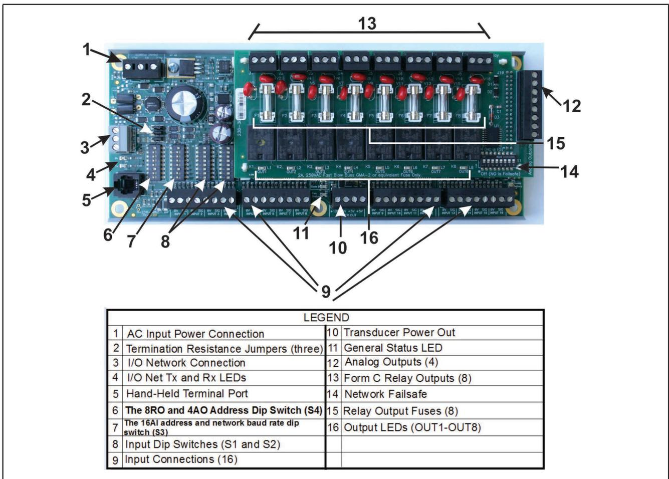
Figure 1-1 - MultiFlex 16 Input Board
