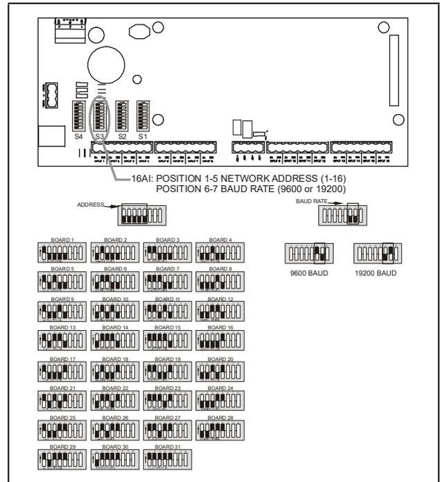
Figure 3-2 - 16 Network ID and Baud Rate Switches
