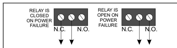
Figure 4-3 - Form C Contact Wiring
