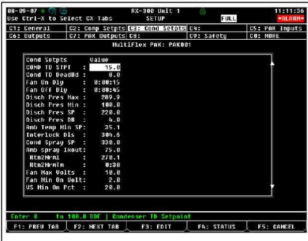
Figure 7-6 - PAK Screen 3: Condenser Setpoints
