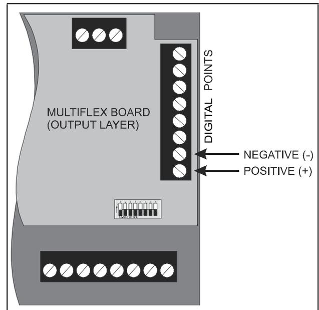
Figure 4-4 - MultiFlex Digital Points
