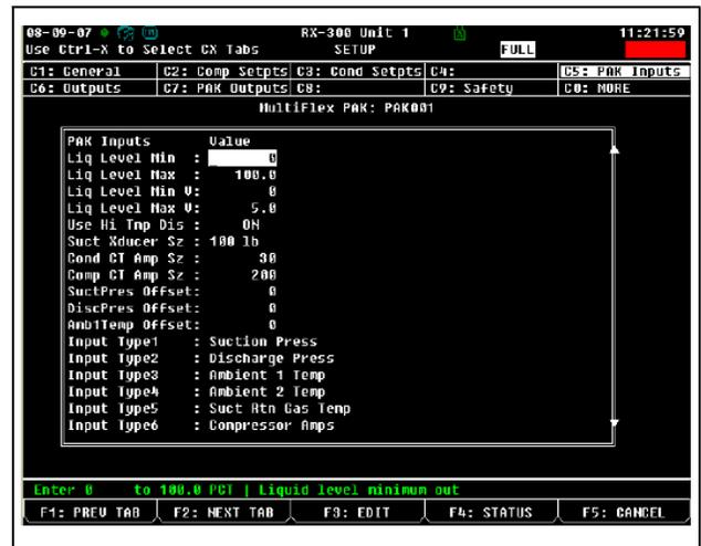
Figure 7-8 - PAK Screen 5: PAK Inputs
