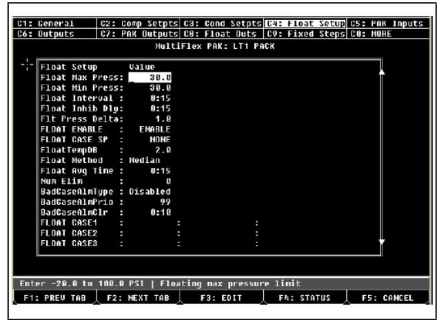
Figure 7-7 - PAK Screen 4: Float Setup Setpoints
