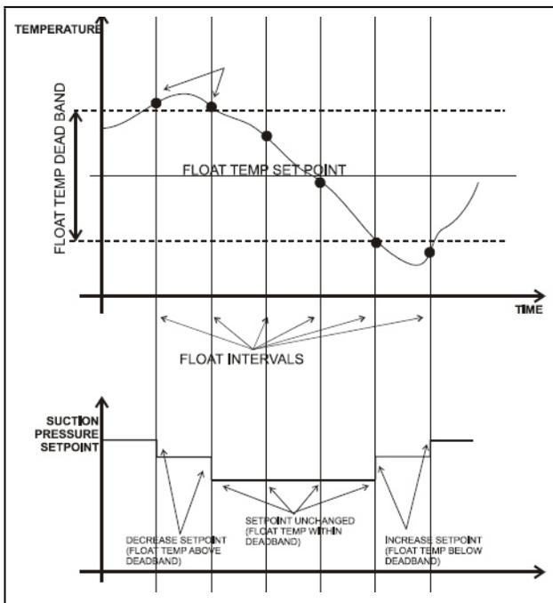
Figure 6-1 - Suction Pressure Setpoint Vs. Float Temperature
