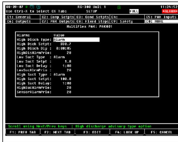
Figure 7-13 - PAK Screen B: Alarms
