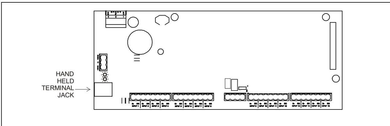
Figure 8-1 - MultiFlex HHT Jack Location
