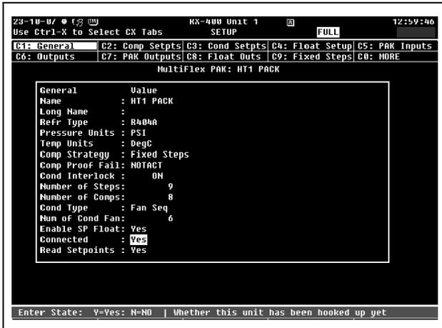
Figure 7-2 - PAK Setup Screen
