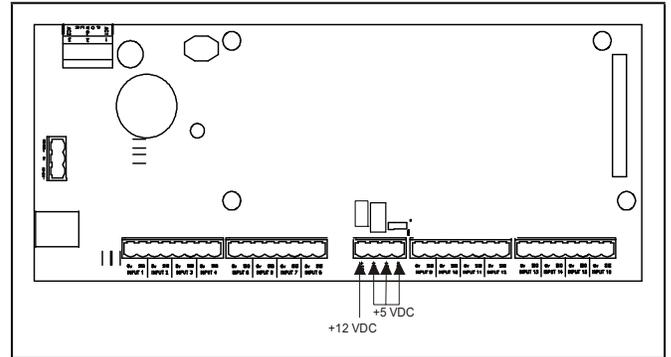
Figure 4-2 - Input Board Power Sources
