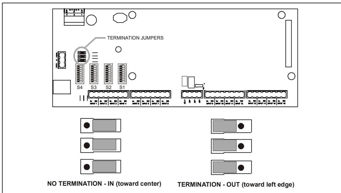
Figure 3-3 - I/O Network Termination Jumper Settings
