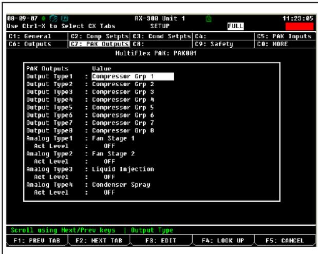
Figure 7-10 - PAK Screen 7: PAK Outputs
