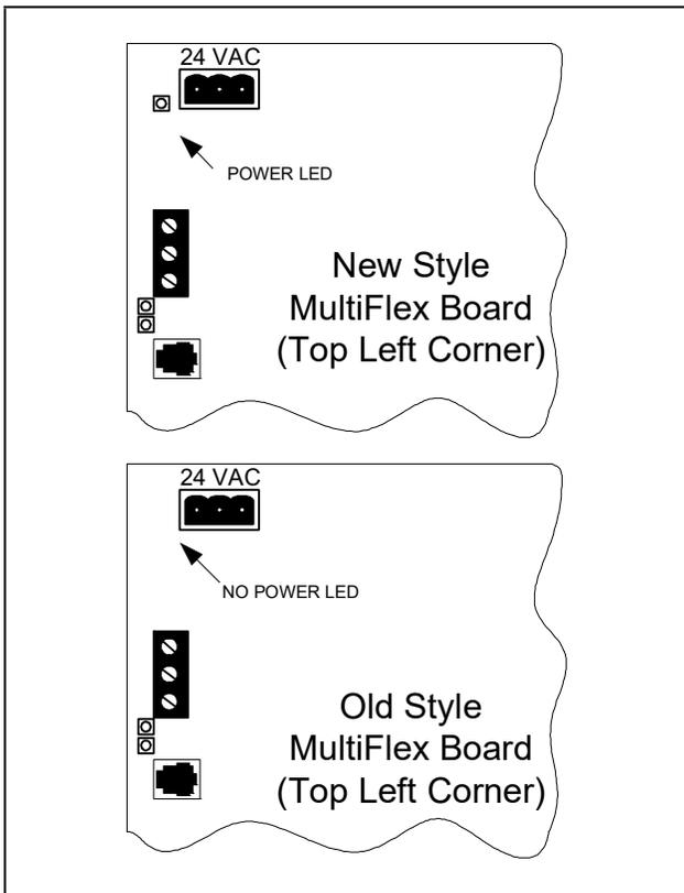
Figure 2-4 - New-Style vs. Old-Style MultiFlex Board
