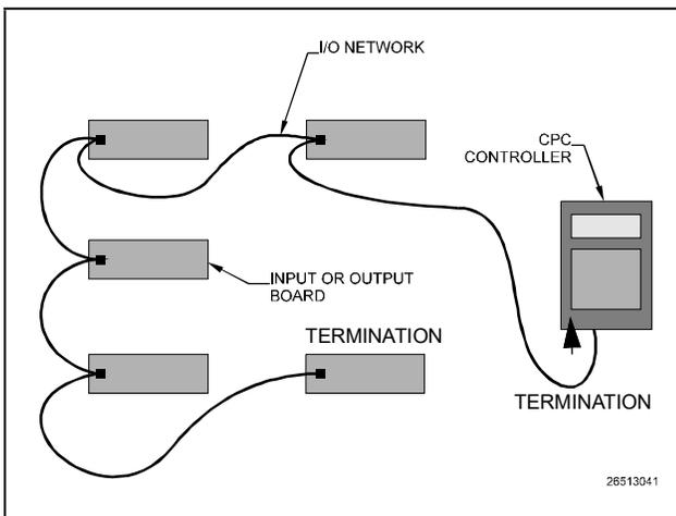
Figure 3-1 - I/O Network Configurations
