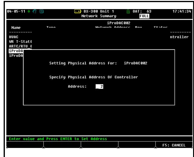
Figure 8-6 - Set the Address of the DAC
