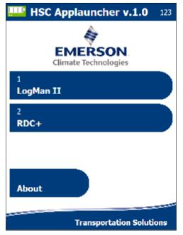
In this example you can press "1" to activate the LogMan Data Retriever Unit software, or "2" to activate the REFCON Data Collector (RDC) software. Also you can "click" the button on the screen.
