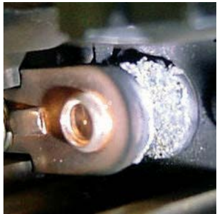
Traditional contactors after 300k cycles
