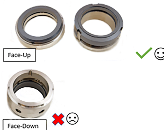
Figure 5-49. Handling Seal Face with Care
