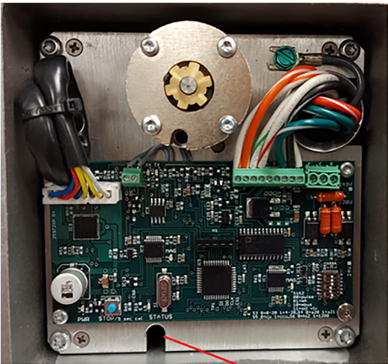
Figure 4-4. Rotation Check. Motor/Brake Shaft Spins Opposite of the Command Shaft
