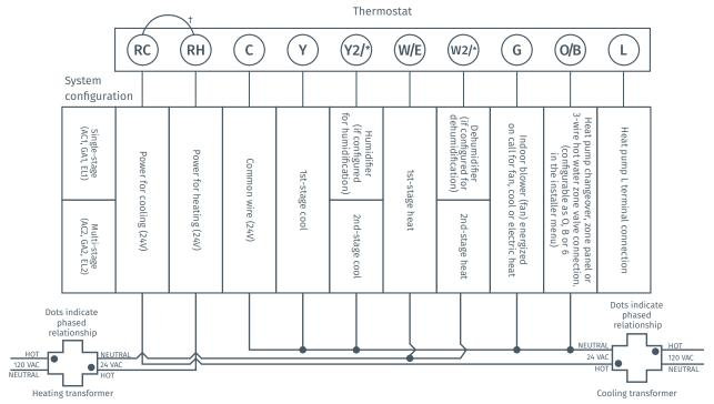
†Two transformers systems (separate RC and RH wires), clip internal RC/RH jumper, located on back of thermostat.
